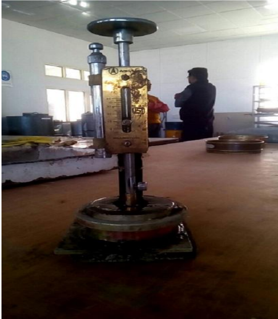
Fig. 3.4: Standard Consistency of Cement/Textile Sludge Paste with Vicat Apparatus
