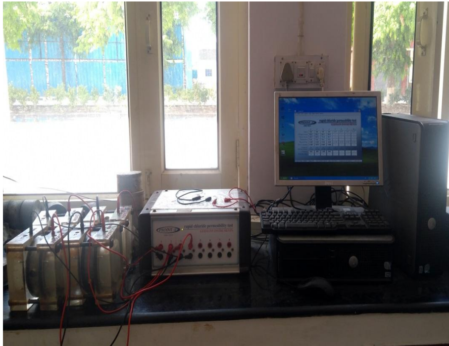
Fig. 3.9: Rapid Chloride Permeability Test Set-up.
