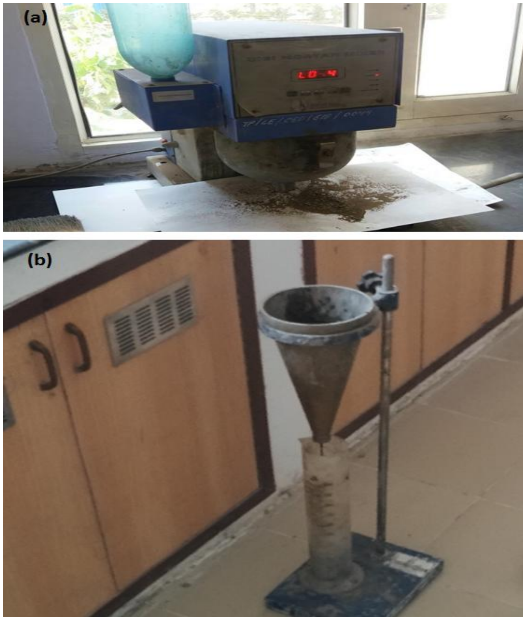
Fig.3.6: (a) Mortar Mixture; (b) Marsh Cone Apparatus to Test Flow Time
