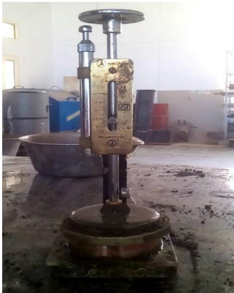
Fig. 3.5: Setting Time of Cement/Textile Sludge Paste with Vicat Apparatus
