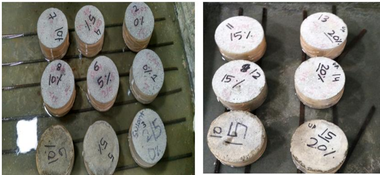
Fig.3.10: Sorptivity Test of Cement/Textile Sludge
