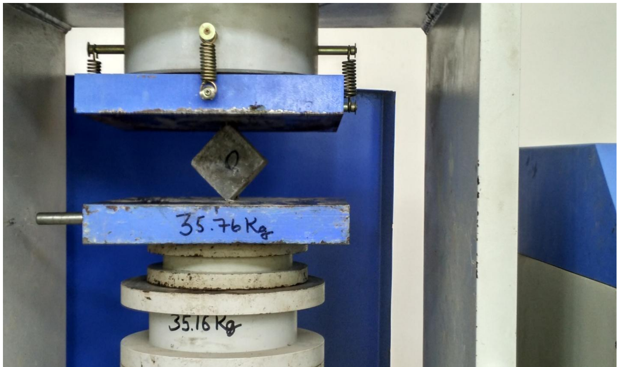
Fig. 3.8: Automatic Compression Testing Machine for Split Tensile Strength Test
