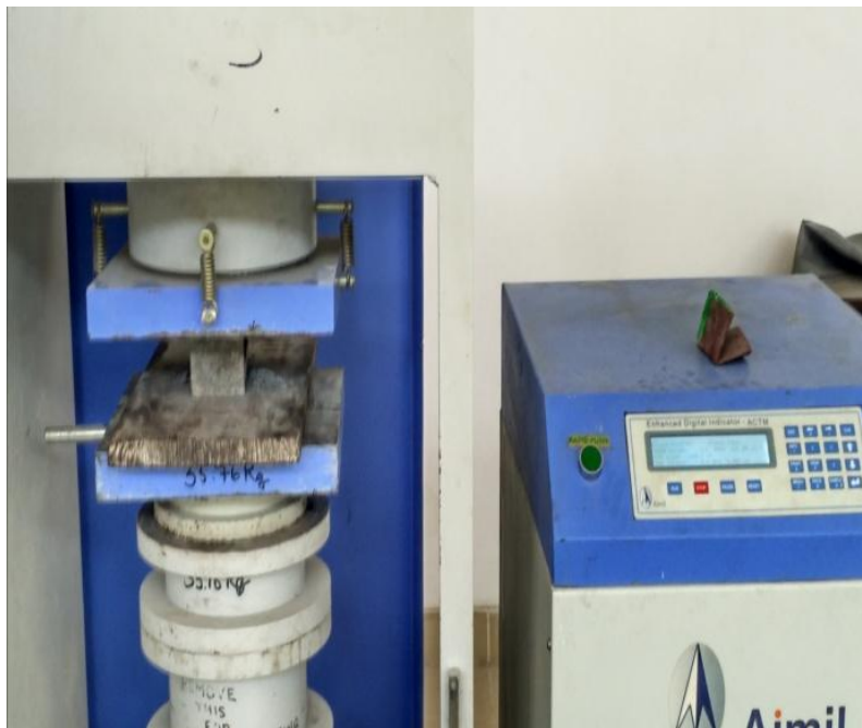
Fig. 3.7: Automatic Compression Testing Machine for Compressive Strength Test
