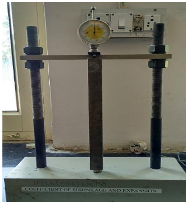
Fig.3.11: Length Comparator to Measure Drying Shrinkage Deformation
