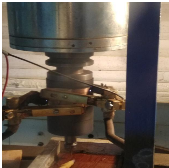
Figure 3.15: Rotary ultrasonic milling of microchannels
