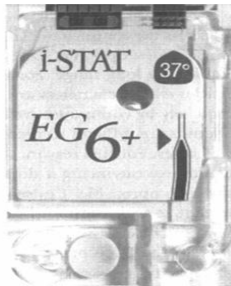
Figure 1.5: Blood sample cartridge using microfluidic channels (The MEMS Handbook 2002)
