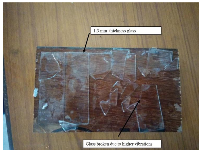
Figure 3.11: Broken glass of thickness 1.3 mm
