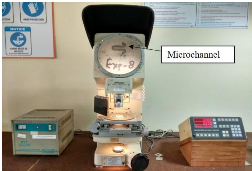
Figure 3.14: Profilometer to measure chipping size
