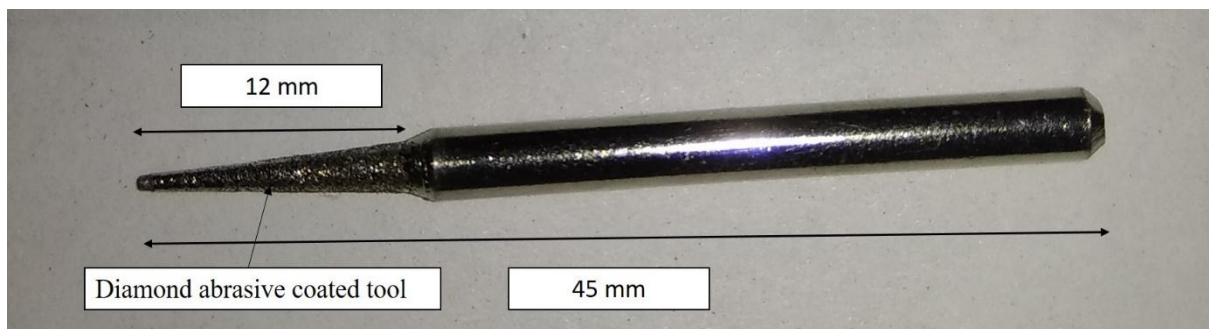
Figure 3.3: Tool used for the fabrication of microchannels
