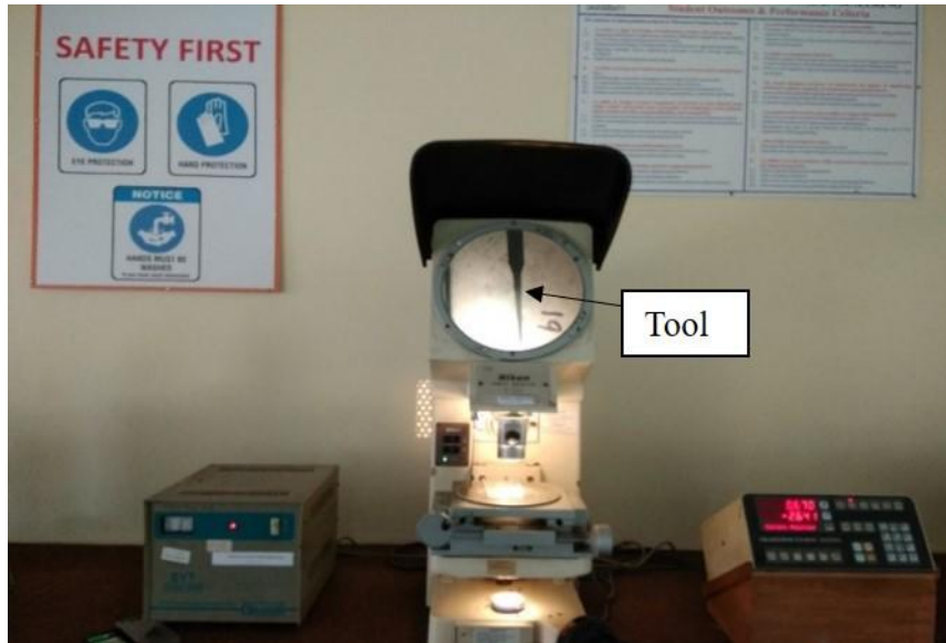
Figure 3.13: Nikon Profilometer used to measure tool wear
