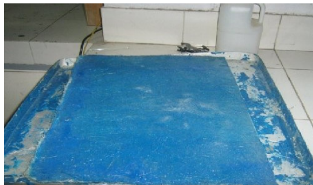
Fig. 4.9 Coated sheets placed for curing
