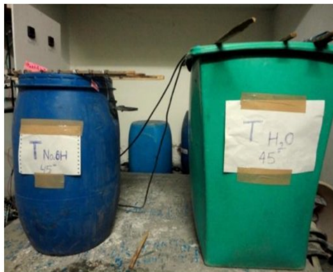
Fig. 4.11 Setup view of the water baths
