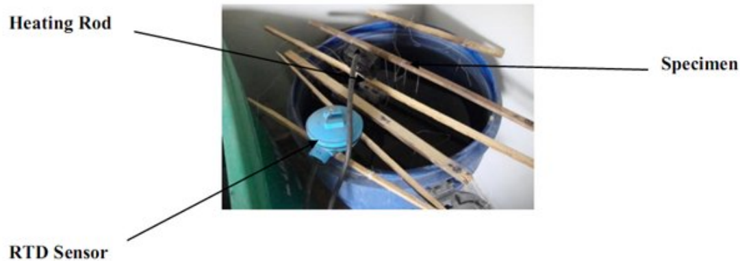
Fig. 4.12 Heating element and RTD sensor in a tank
