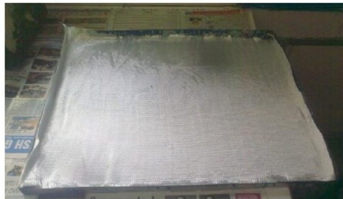
Fig. 4.3 Uncoated E glass fiber mat used for making specimen
