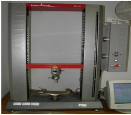
Fig. 4.17 Three point bend test machine
