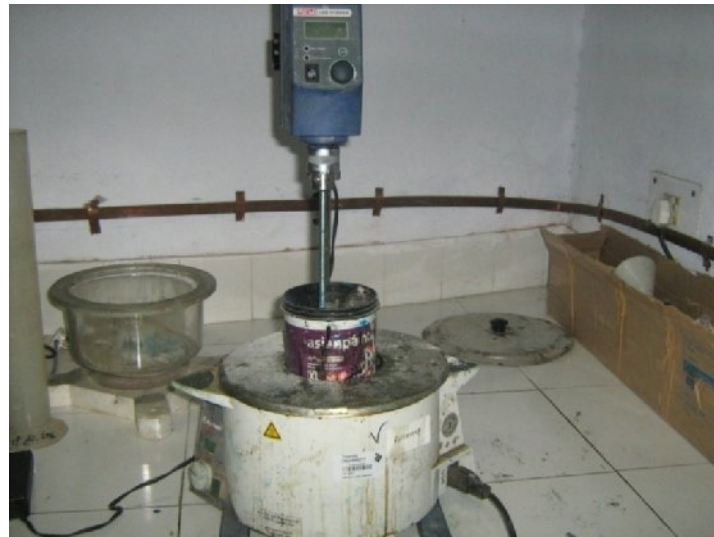
Fig. 4.5 Oil bath setup with mechanical stirrer
