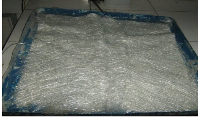
Fig. 4.4 Uncoated C- glass fiber mat used for making specimen
