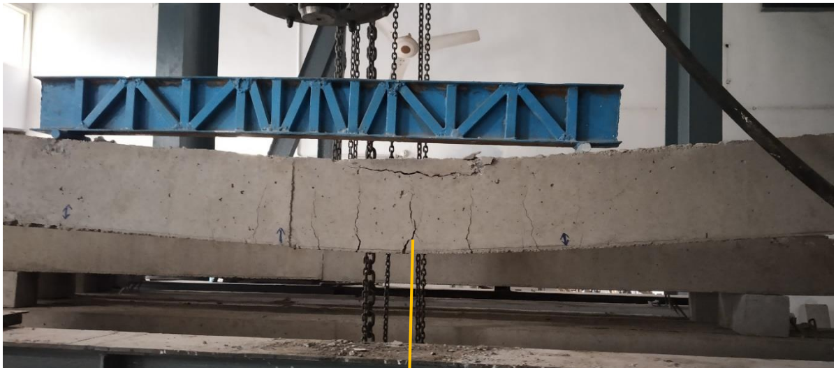
Figure 4.2 crack pattern in control beam
