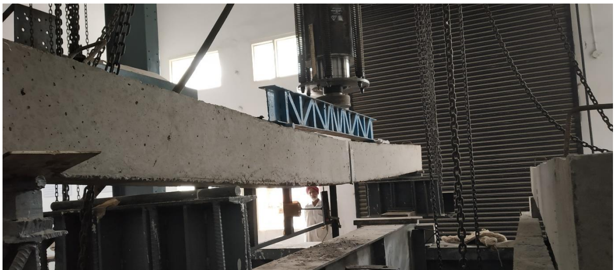
Figure 3.2- Two Point Loading Testing Arrangement
