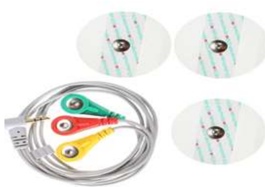
Figure 1.5: Surface electrode with EMG cable [12].
