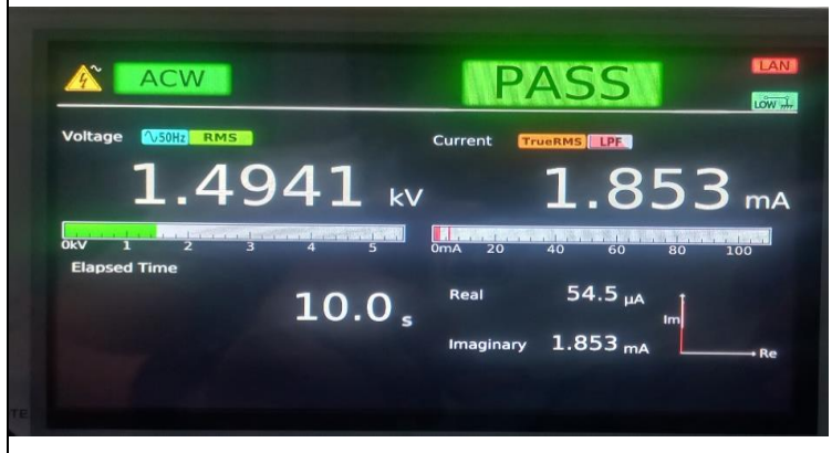
Figure 4.18 High voltage test results
