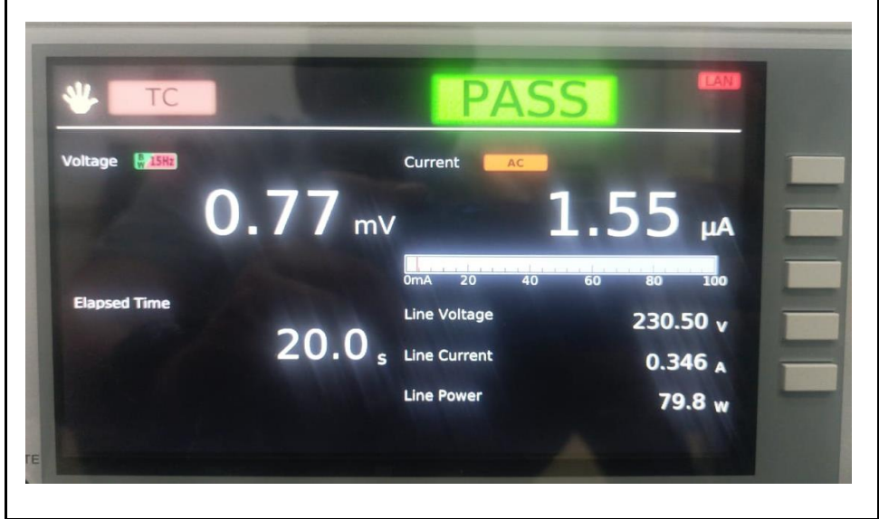
Figure 4.17 Leakage Current test result
