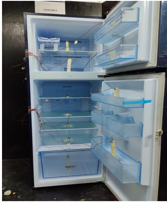
Figure 3.10 Thermocouples placement in frost-free refrigerator for Temperature rise testing.
