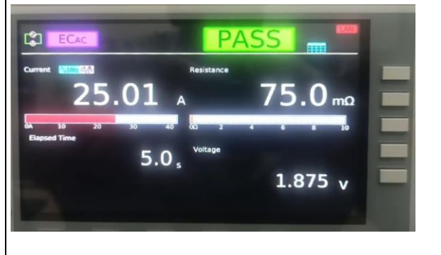
Figure 4.19 Earth Continuity test result
