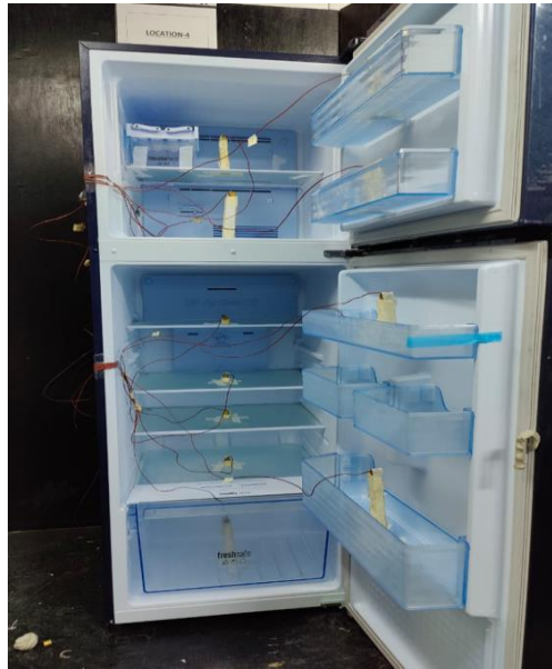
Figure 3.94 Thermocouples placement in the frost-free refrigerator for notch and continuous testing
