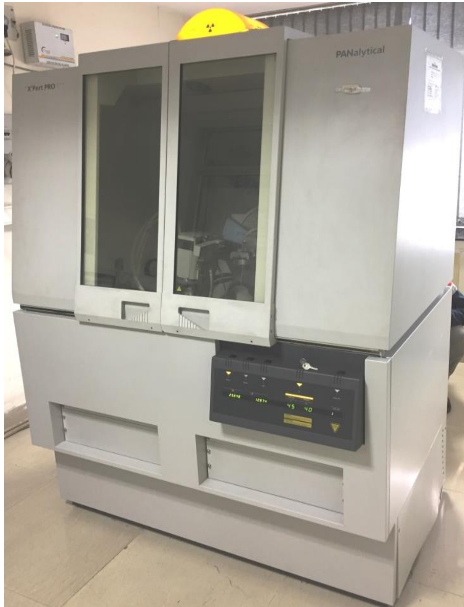
Figure 3.3 Phillip X'Pert X-ray diffractometer (Model: PW 1710)
