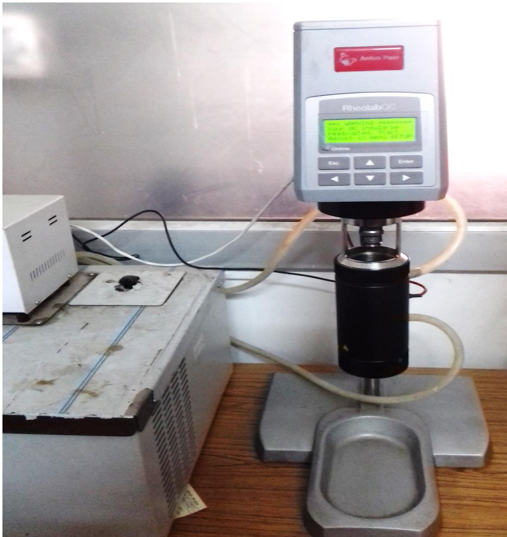
Figure 3.5 Rheometer (Rheolab QC Anton Paar) used for rheological experimentation
