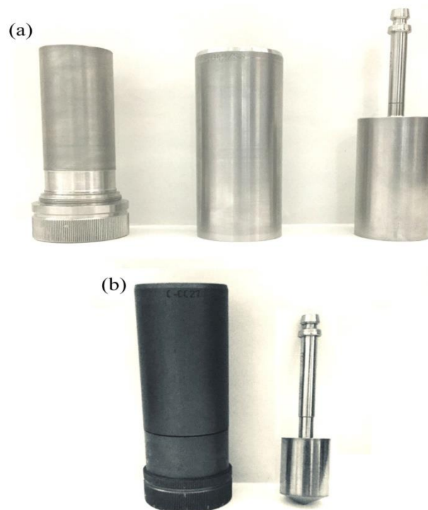
Figure 3.4 (a) Cylinder cup and rotating bob assembly (b) Cone and Cylinder rheometer assembly
