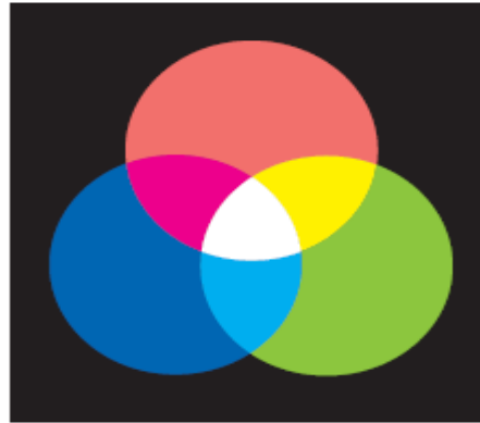
Fig: 3.2 Projections of three lamps with the colors red, green and blue onto a wall in a dark room
