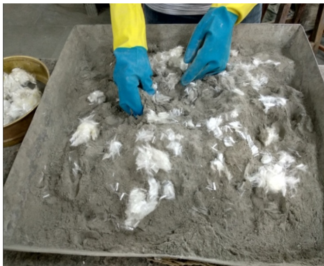
Fig 3.7 Mixing of PVA fibers in laboratory
