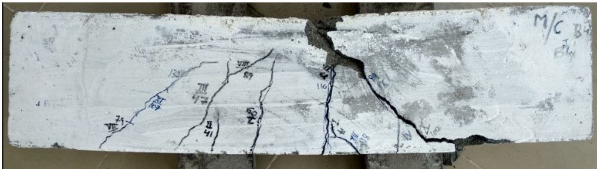
Fig 4.9 Cracking pattern of beam repaired with Micro Concrete
