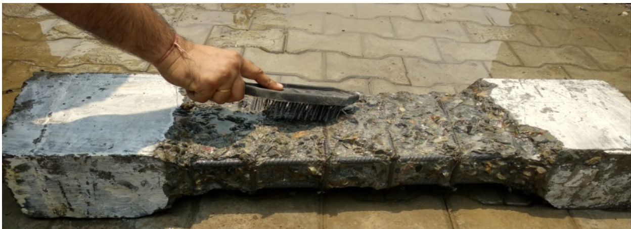
Fig 3.9 (a). Removal of dust with wire brush
