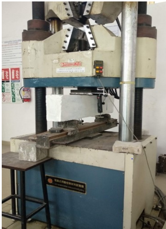
Fig 3.5 Test setup for single point loading
