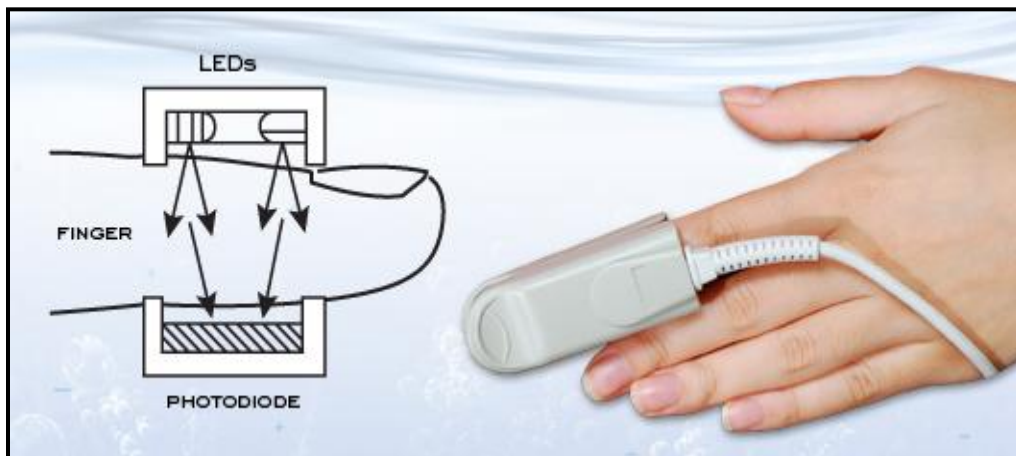
Figure 3.7: Picture representing the functioning of probe in Pulse-oximeter
