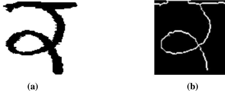
Figure 3.2 A sample handwritten Gurmukhi character ( ਕ ): (a) Digitized image, (b) Thinned image
