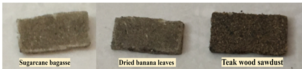
Figure 3.8 Developed microwave absorber samples using sugarcane bagasse, dried banana leaves, and teak wood sawdust
