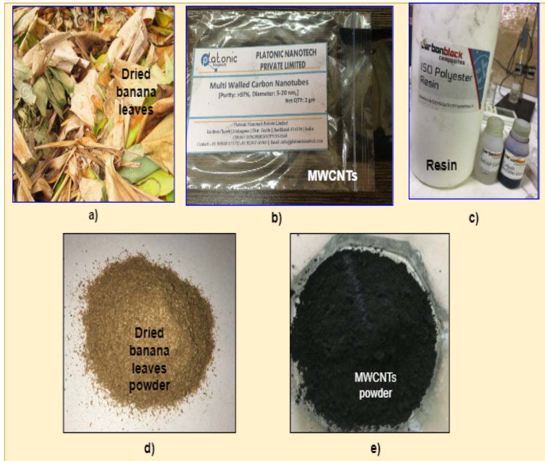
Figure 4.1. Primary raw materials used for fabrication MA (a) Banana leaves waste (b) MWCNTs (c) polyester resin (d) powder form of banana leaves and (e) MWCNTs powder
