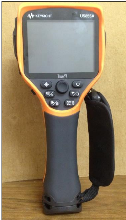
Figure 3.7: TrueIR Thermal Imager (Keysight Technologies).
