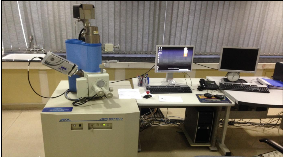
Figure 3.13: SEM set-up used for microstructural characterization in the present work.
