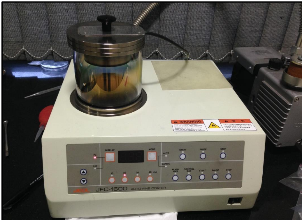
Figure 3.11: Auto Fine Coater used for coating the bone specimens.
