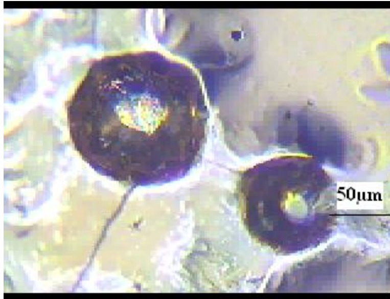
5.22 Micro structure of 7.5% Calcite with DC(-) at 200 X
