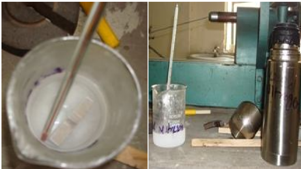
Fig 5.14 Specimen Dipped in Liquid Nitrogen and Temperature measured with thermometer
