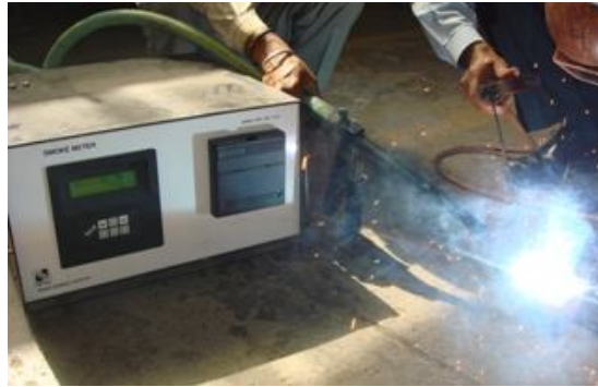
Fig 4.13 Smoke Testing of Welding Electrode by Smoke Meter
