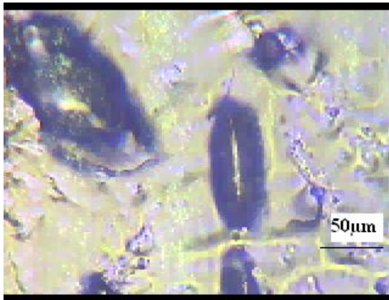
5.27 Micro structure of 20% Calcite with DC(-) at 200 X
