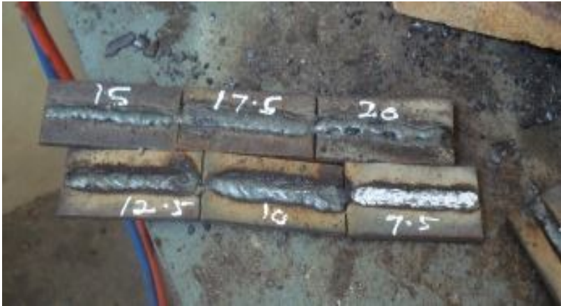
Figure 5.1 Weld bead obtained on Welding with AC
