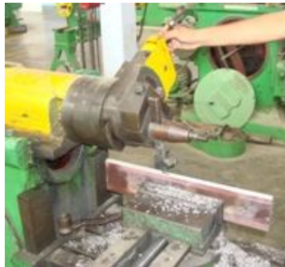
Fig 4.10 Cutting V Groove on Plate for Tensile Specimen Formation
