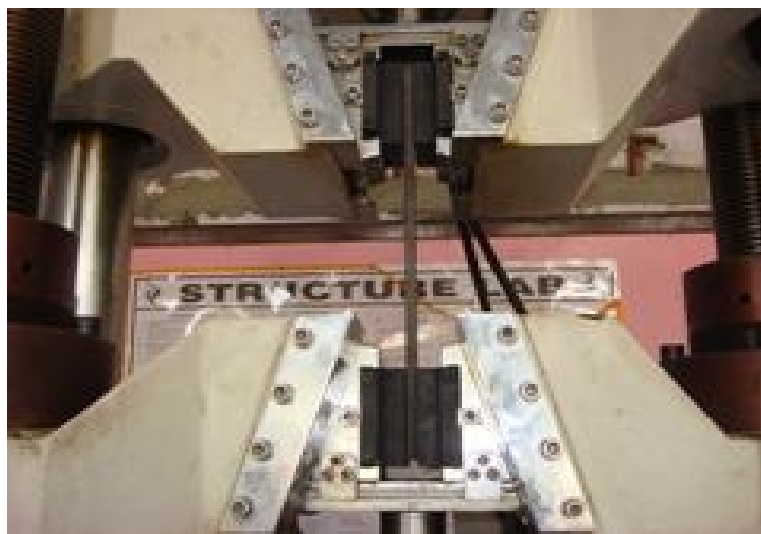
Fig 5.9 Tensile Weldment Specimen Gripped on UTM
