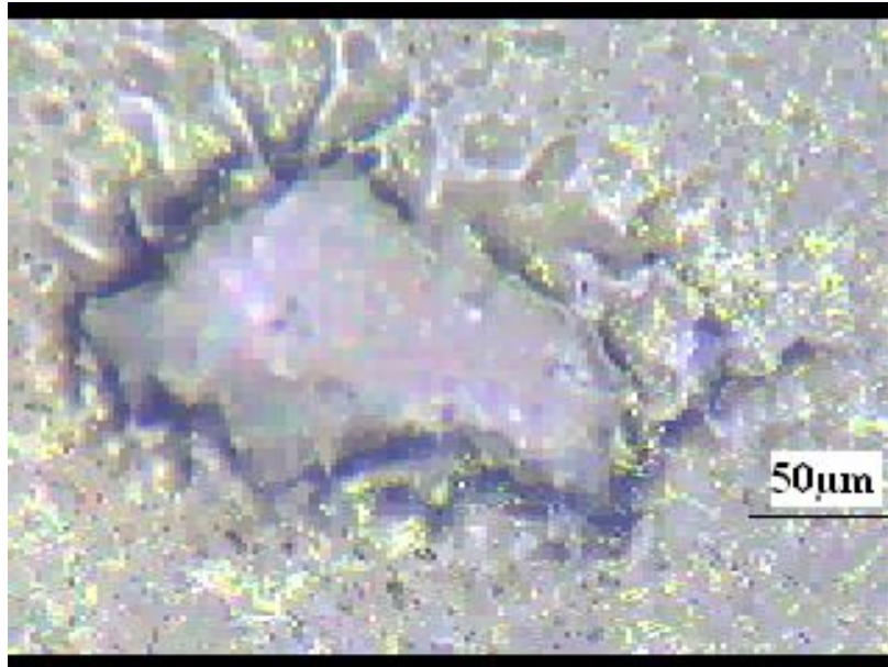
5.20 Micro structure of 17.5% Calcite with AC at 200 X
