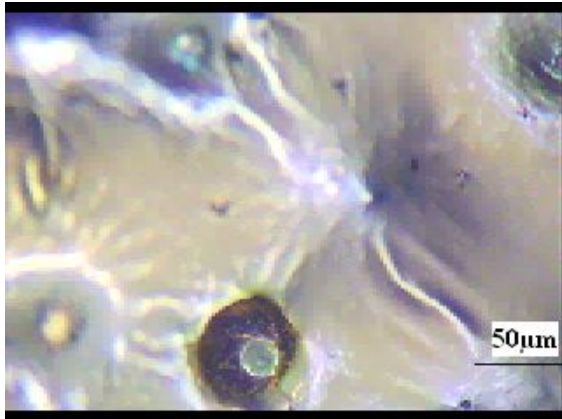
5.24 Micro structure of 12.5% Calcite with DC(-) at 200 X
