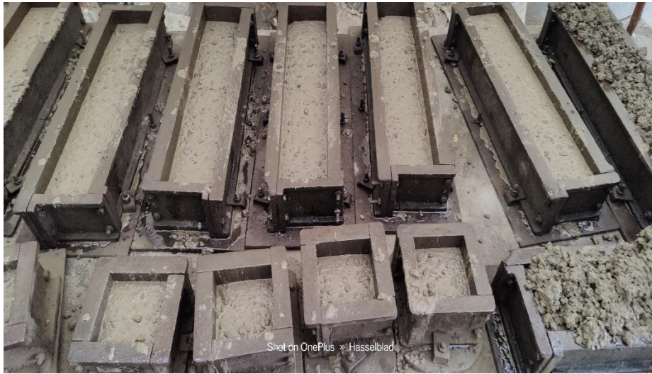
Figure 3.23 Concreting of Beams and Cubes
