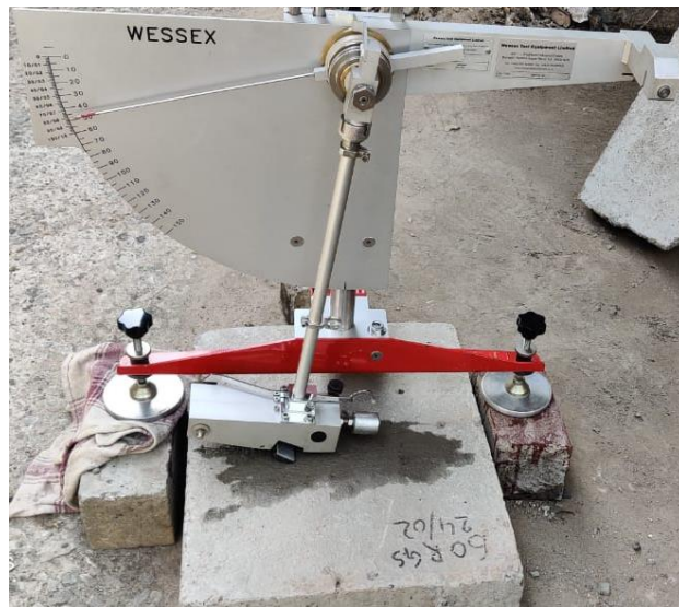
Figure 4.30 BPT on wet surface of slab specimen
