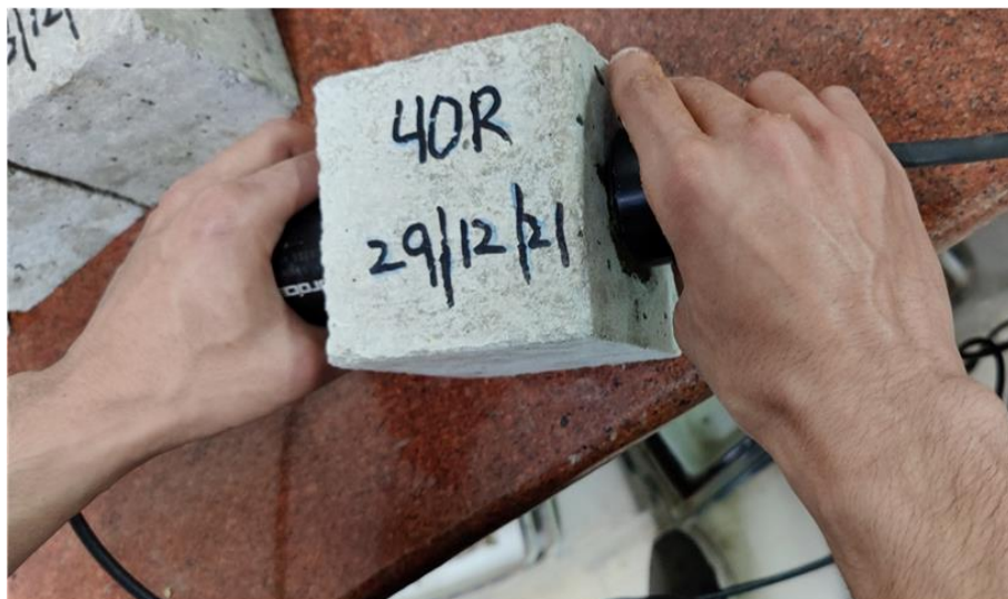
Figure 4.39 Testing of concrete specimen using UPV
