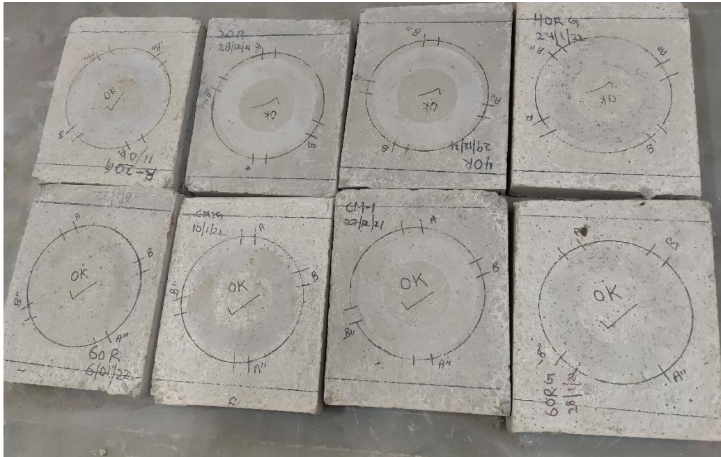
Figure 4.23 Samples of various concrete mixes tested for abrasion resistance
