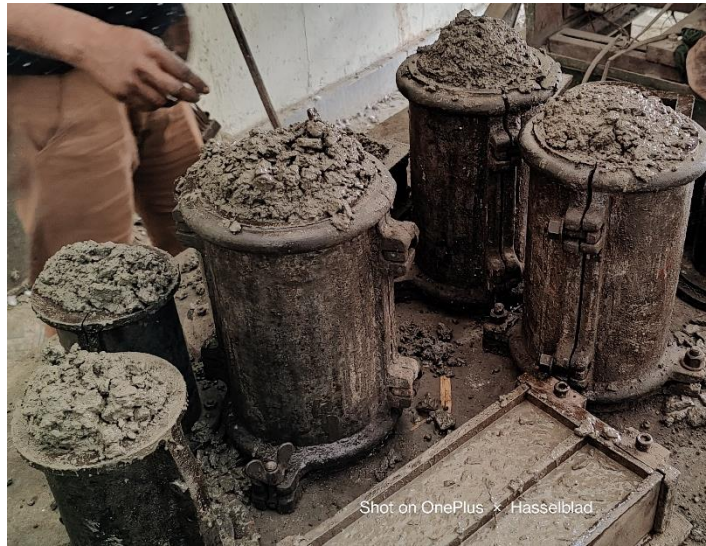
Figure 3.24 Concreting of Cylinders and Prisms
