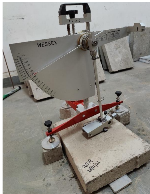
Figure 4.29 BPT on Dry surface of slab specimen
