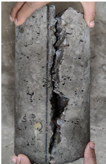
Figure 4.18 Top view of specimen failed in split tensile test
