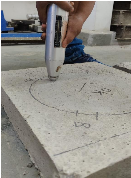
Figure 4.35 Vertical impact on the horizontal surface of the concrete slabs
