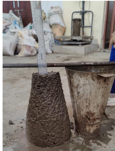
Figure 4.3 Slump of normal concrete mix
