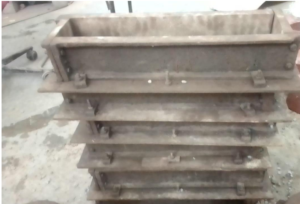
Figure 3.20 Prepared moulds of Beams
