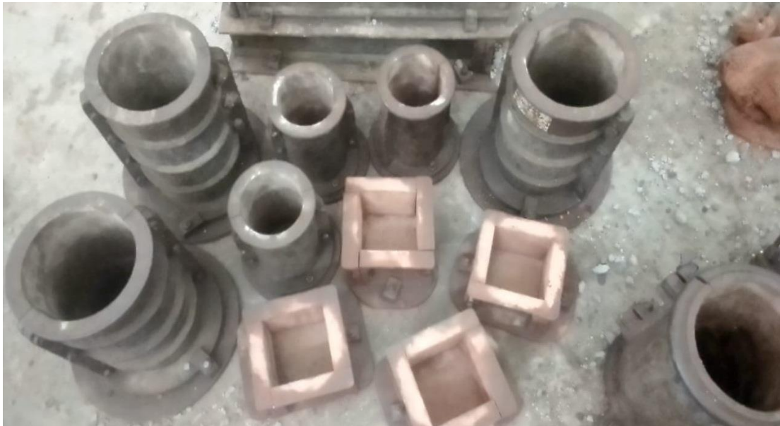
Figure 3.19 Prepared moulds of Cylinders and Cubes
