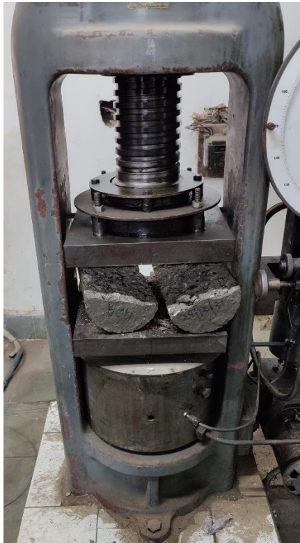
Figure 4.17 Failure of the specimen during loading
