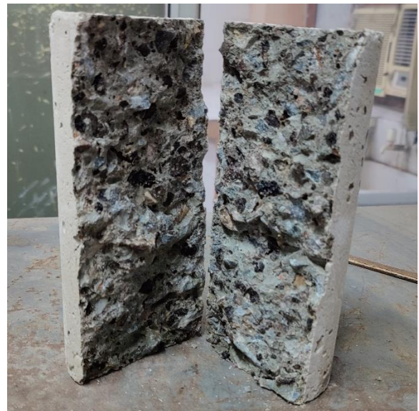
Figure 4.19 Front view of specimen failed in split tensile test
