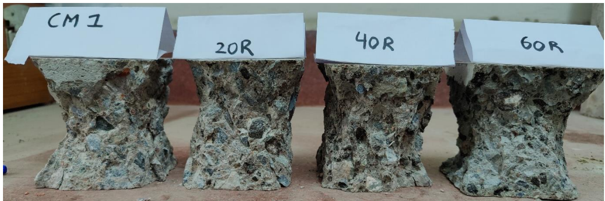
Figure 4.8 Failure Pattern of various concrete mixes under compression after 28 days
