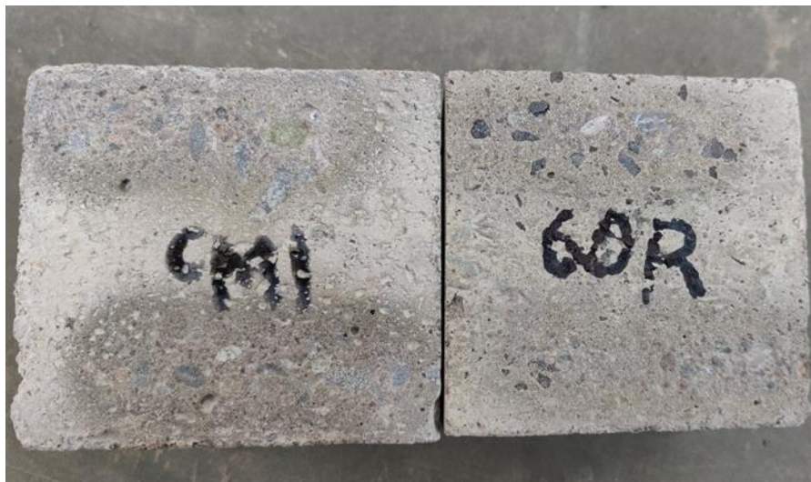
Figure 4.26 Various concrete cubes after sand blasting
