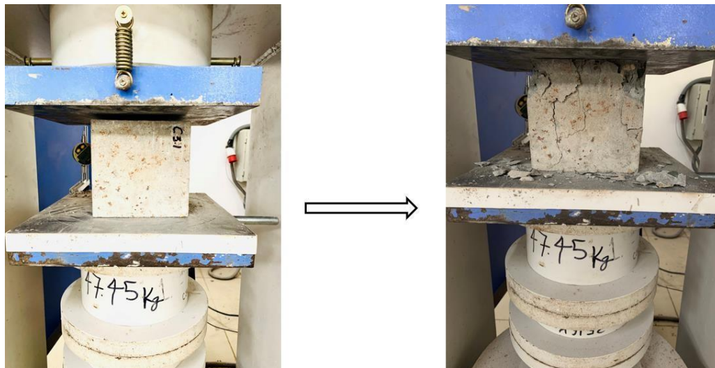
Fig. 4.20 Compressive strength test
