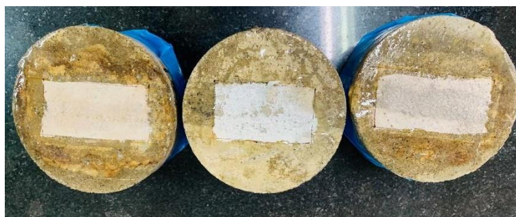
Fig. 4.22 Surface of epoxed crack exposed to water for water sorptivity analysis
