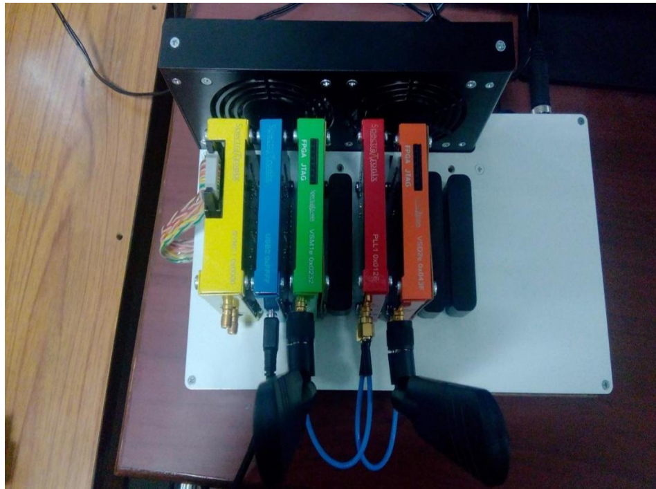
Figure 5.5 Connections of C700 Modules
