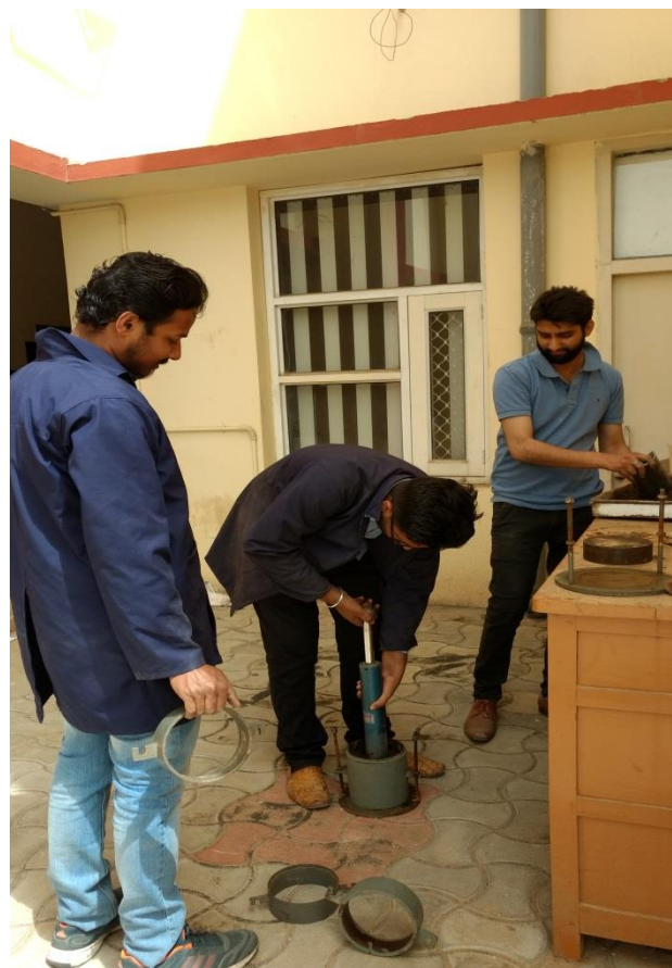
Figure 4.5: Light Compaction Test
