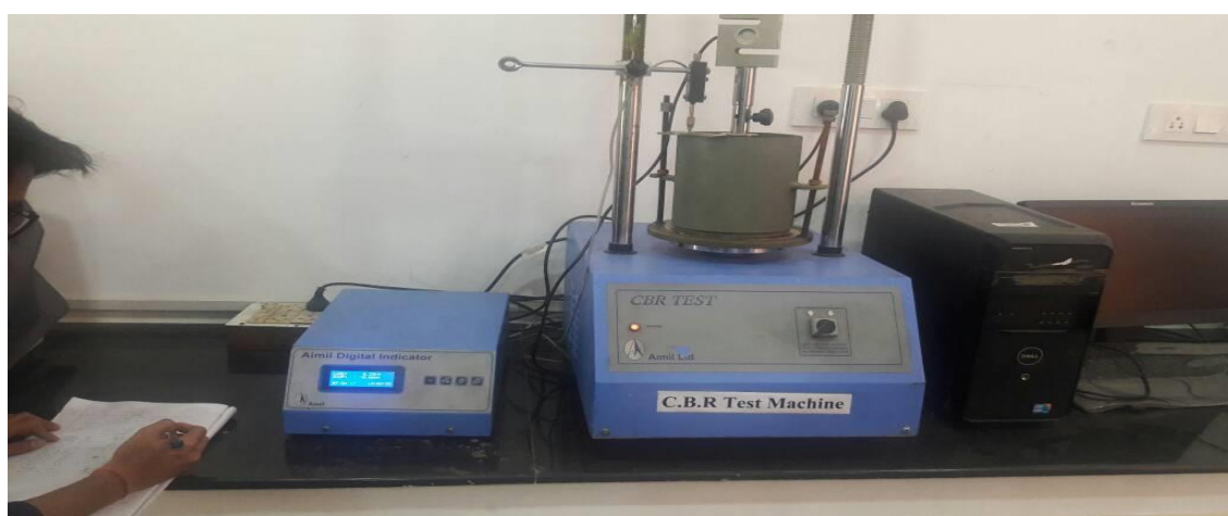
Figure 4.6: CBR testing of soaked sample
