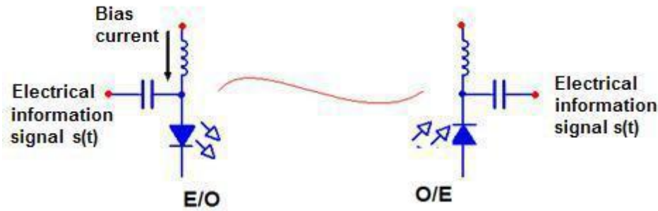
Fig. 1.11 Schematic Intensity Modulation and Direct Detection.
