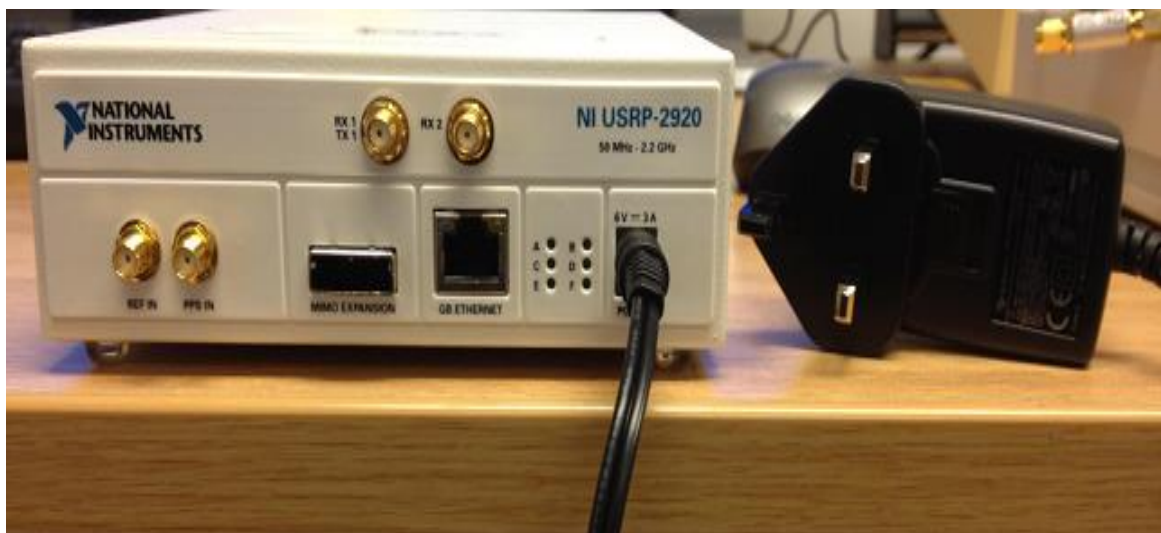
Figure 4.3: Power connections to the USRP kit
