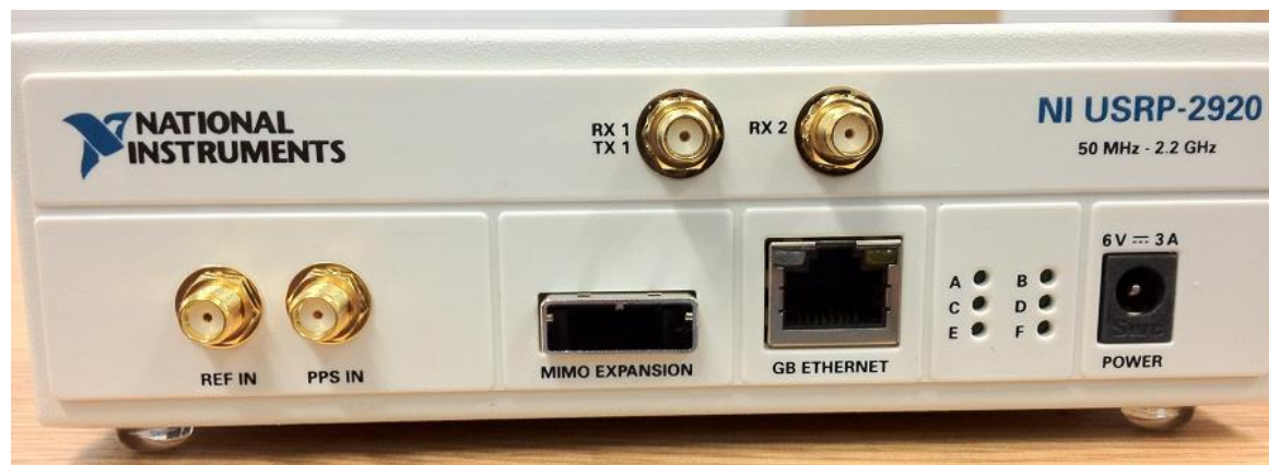
Figure 1.7: Front Panel of NI-USRP
