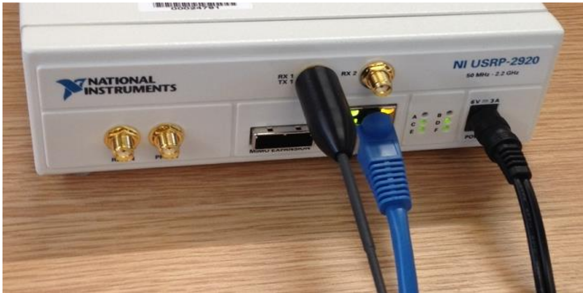
Figure 4.4: Ethernet cable and antenna connections to the USRP kit
