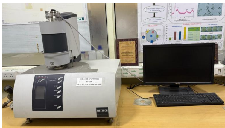
Fig. 2.3: Actual photograph of the experimental setup used for TGA measurements
