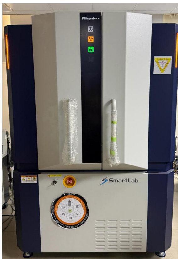
Fig. 2.4: Actual photograph of the experimental setup used for XRD measurements
