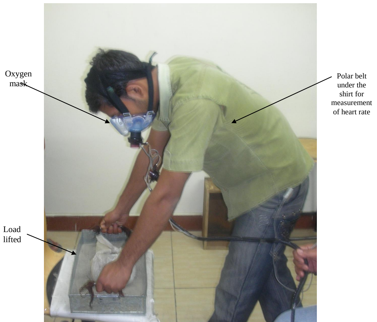
Figure 5.1: Worker involved in manual lifting task using COSMED pulmonary equipment
