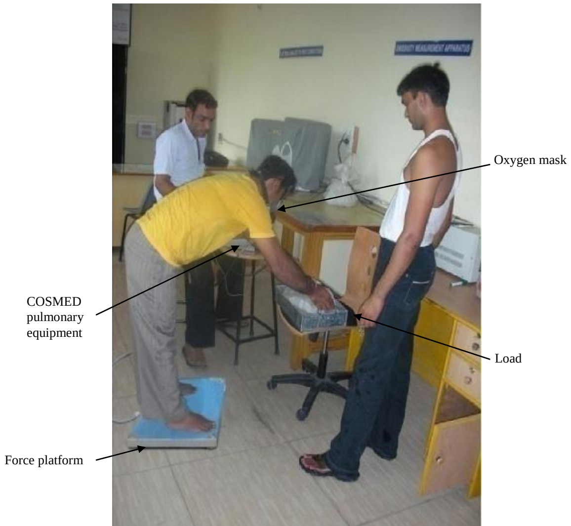
Figure 8.1: Experimental Set up with Kistler force platforms and COSMED pulmonary function equipment
