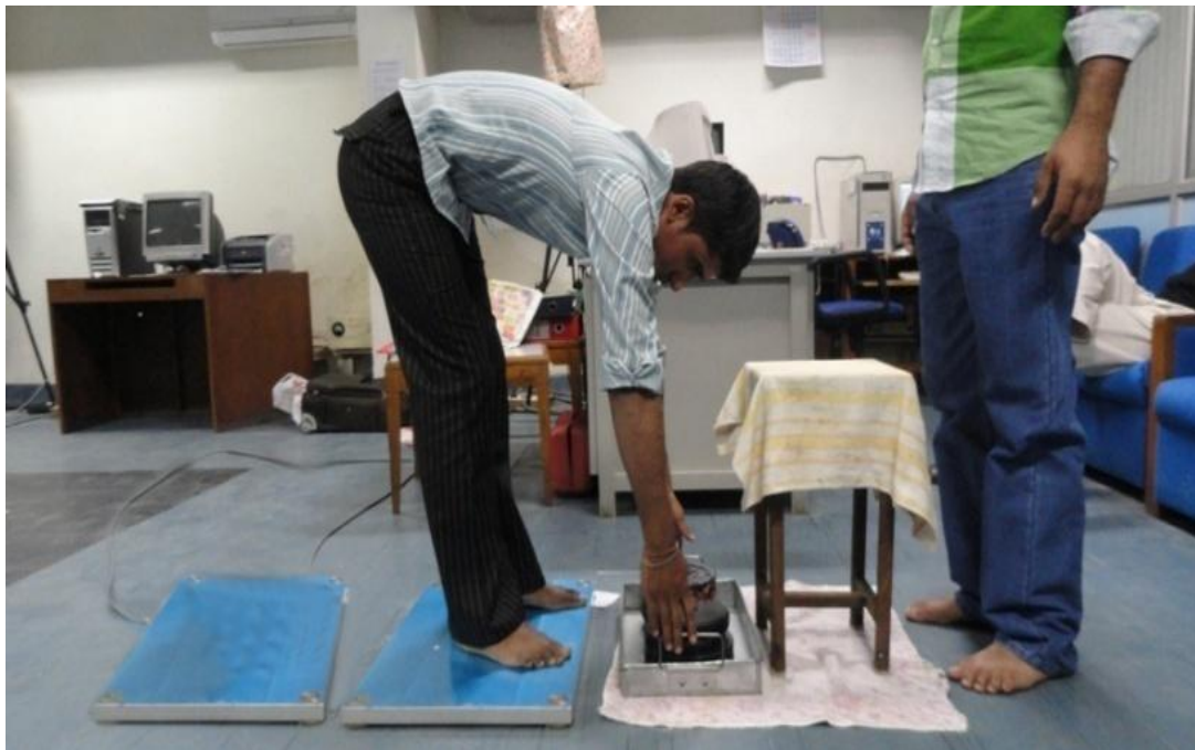
Figure 7.1: Experimental Set up with Kistler force platforms
