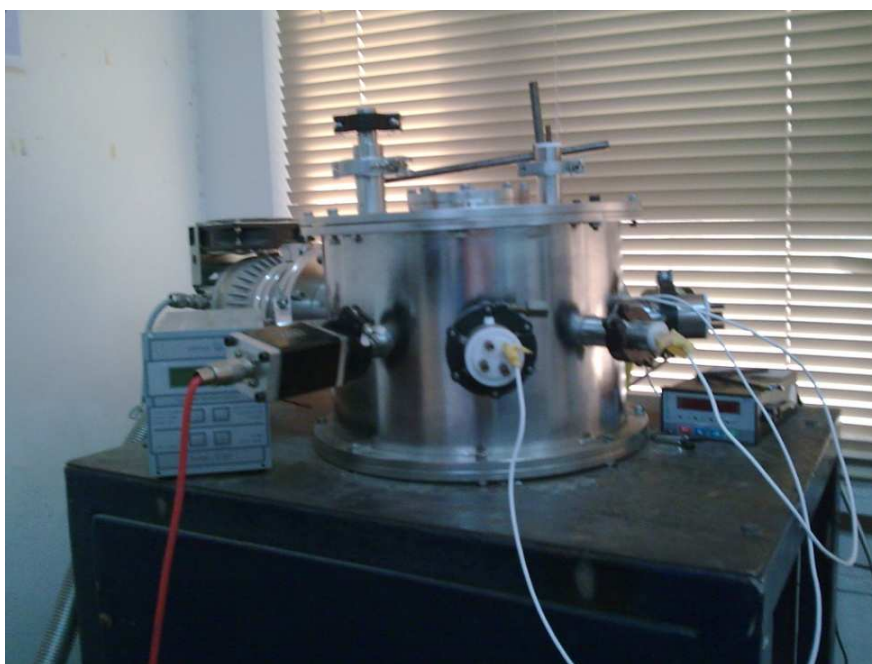
Fig.4.2: Experimental set-up for field emission studies.
