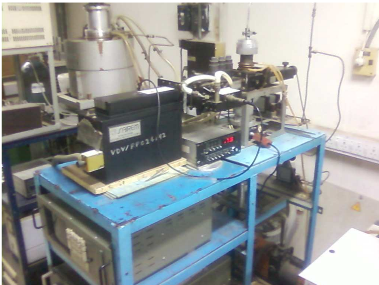
Fig.2.2: Front view of MPECVD set up.
