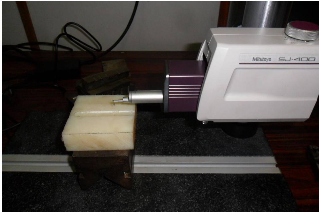
Figure: 3.5 Experimental devices for measurement of surface roughness [Metrology lab]
