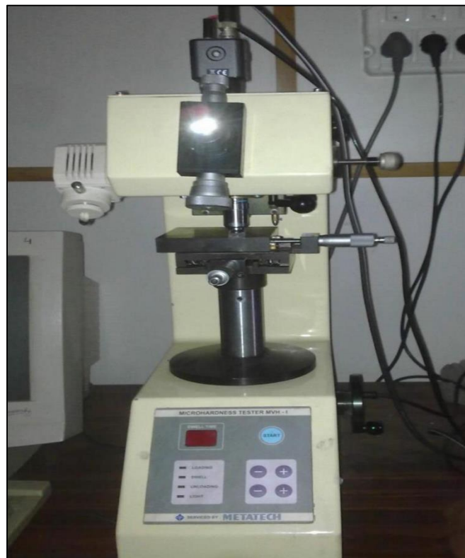
Figure 3.5 Micro hardness testing machine (Model: MVH2) (Courtesy: Measurement and Control Lab,Thapar University)
