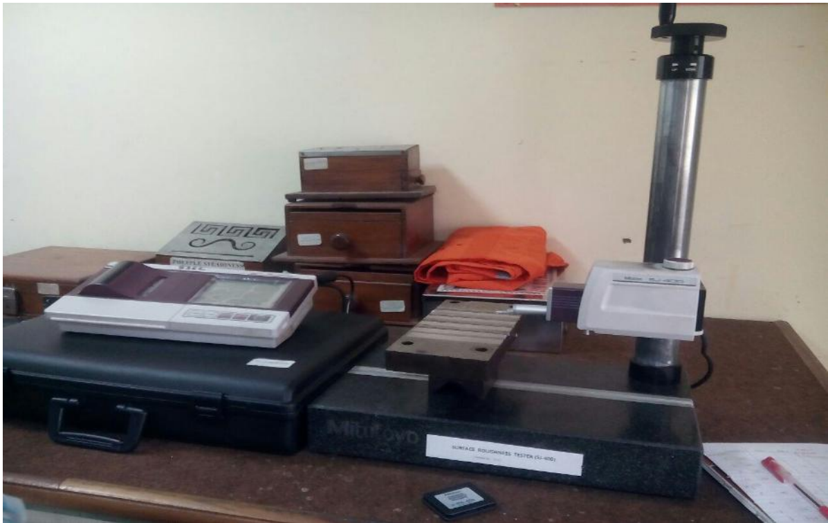
Fig. 3.7 Surface Roughness Tester (Surftest SJ-400)
