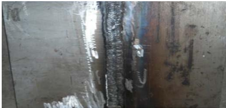
Fig.5.15 Welded Specimen with 6 mm buttering layer
