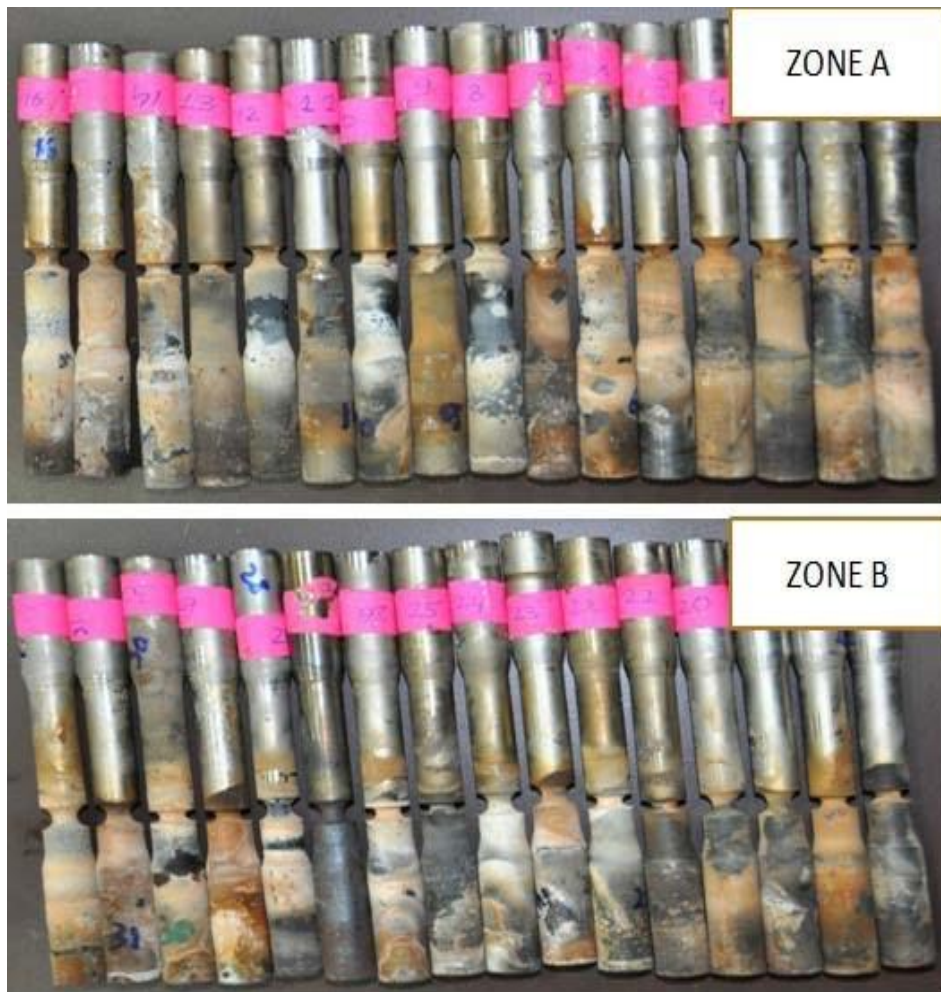
Fig.5.27 Tensile Specimens after Thermal Fatigue
