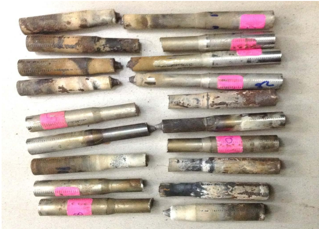
Fig.5.28 Fractured Specimens after Thermal Fatigue
