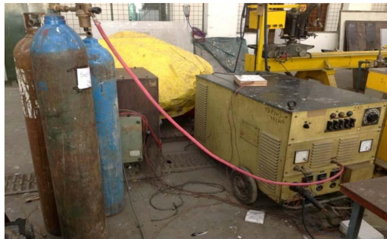
Fig.5.5 GTAW Welding Machine
