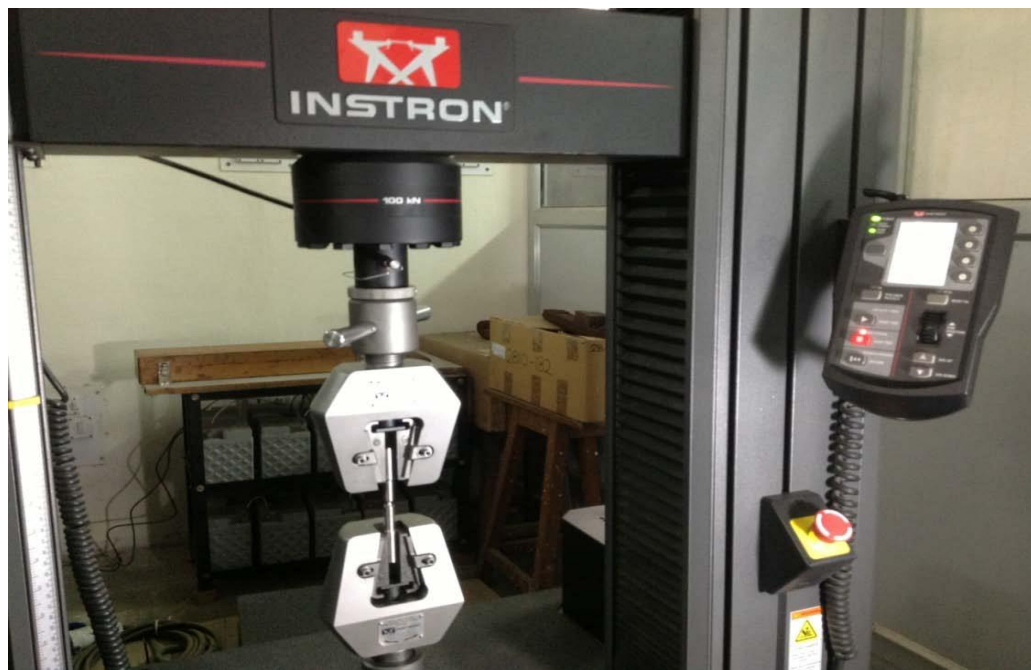
Fig.5.25 Tensile Testing Machine loaded with sample
