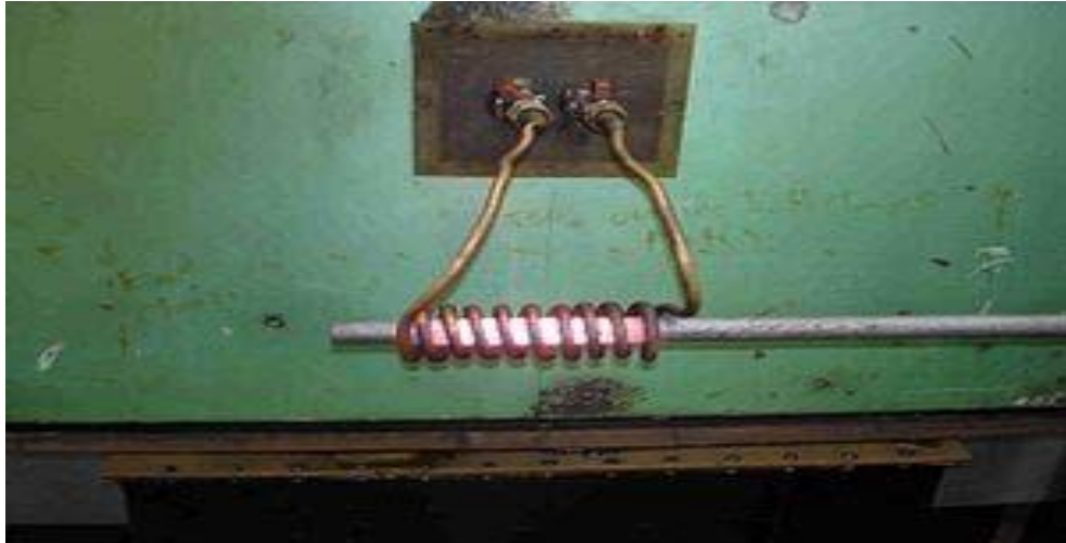
Fig.4.3. Induction heating of 25 mm metal bars using 15 kW at 450 kHz. [116]
