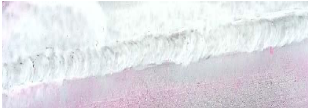
Fig.5.17 Weld bead profile after application of developer
