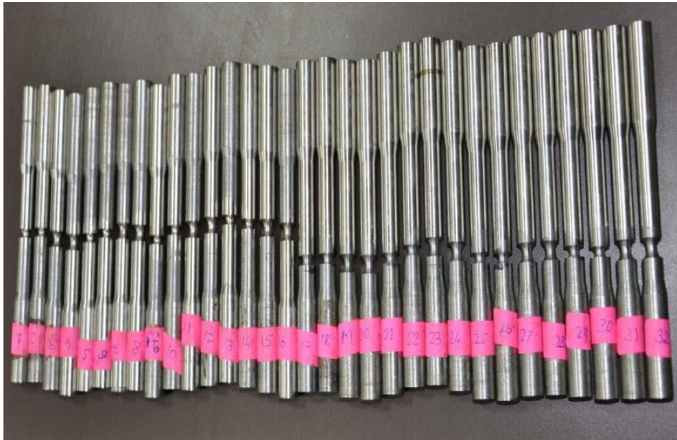
Fig.5.26 Tensile Specimens before Thermal Fatigue
