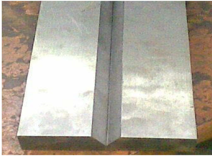
Fig. 5.2 Plates with V groove
