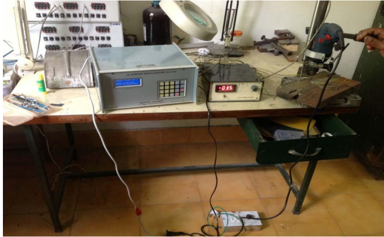
Fig.5.7 Strain measurement setup
