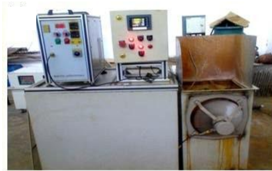
Fig. 4.10 Overview of the Thermal Fatigue Test Rig
