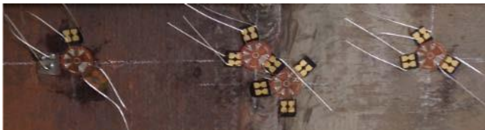
Fig.5.6 Placement of Strain Gauges in different Zones.
