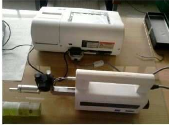
Figure 4.2: Tokyo Seimitsu Surfcom 130A type instrument for Surface Roughness Testing.
