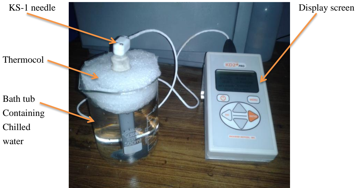
Figure 5.12 Measurement of thermal conductivity using KD2 Pro
