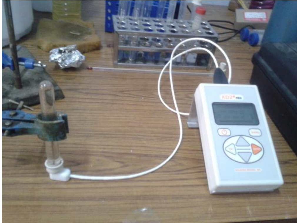
Figure 4.2 KD2 Pro thermal properties analyzer
