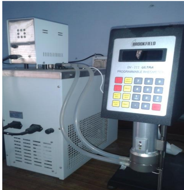
Figure 5.13 Measurement of viscosity by Brookfield Rheometer (LV DV-IIIICP)
