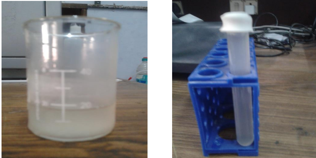
Figure 5.11 \text{Al}_2\text{O}_3/\text{R-11} nanorefrigerant after sonication
