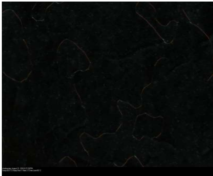
Figure 4.2 Texture of 6OCB-Fe mixture under polarizing microscope at 10x (a) 0 (b) 1.8 (c) 2.0 (d) 4 (e) 8 (f) 12 V at 65°C. Cross arrow indicates the position of polarizer and analyzer.
