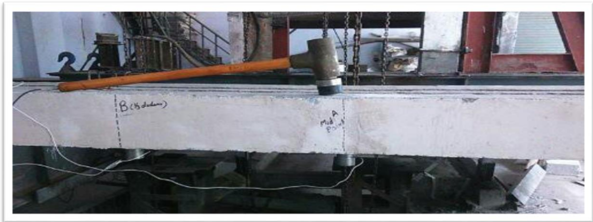
Figure 3.10 Accelerometer placed below at centre and one third position of beam
