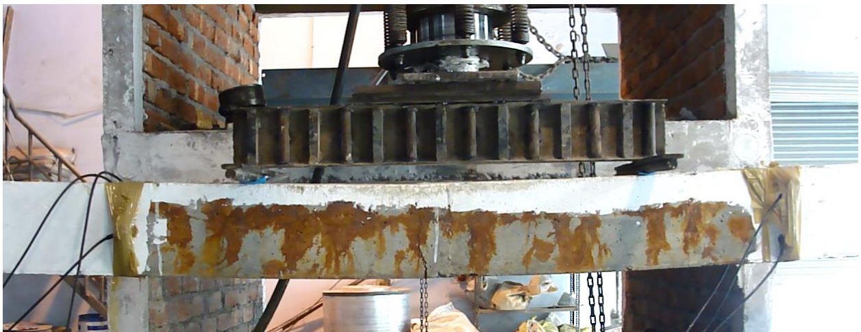
Figure 4.17 C-20 Beam showing large vertical crack near the centre of beam
