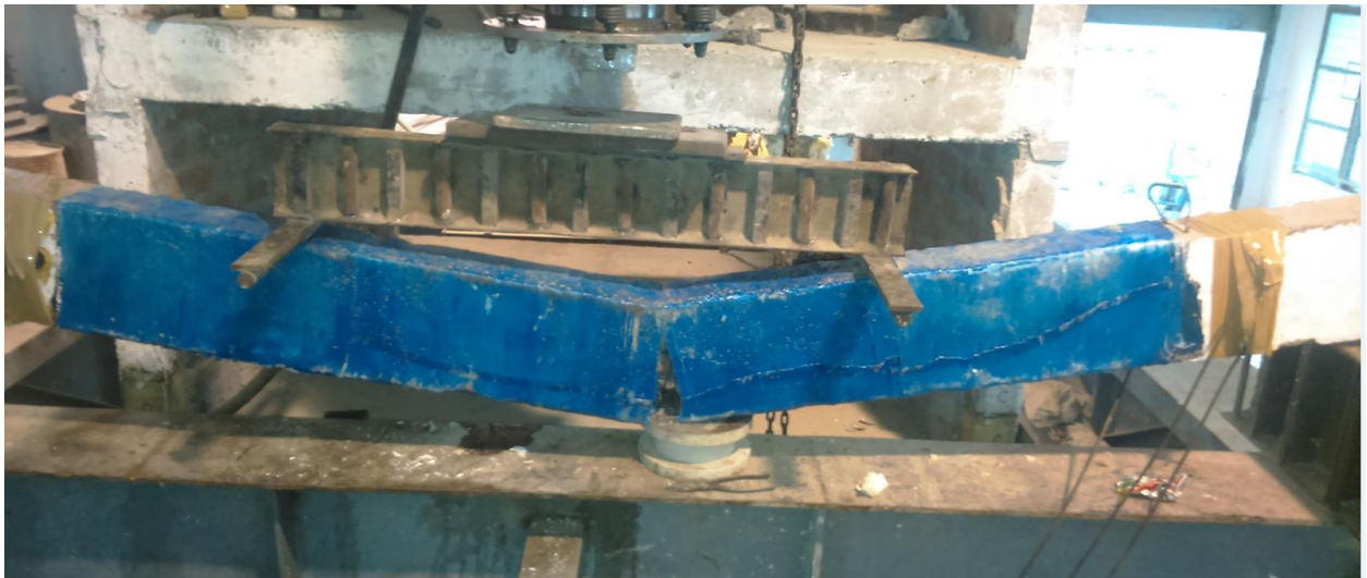
Figure 4.28 F-60 Beam cracked from the centre
