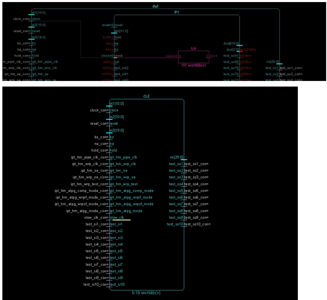
Figure 4.36 Schematic showing all the scan signals
