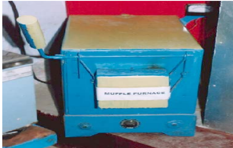
Plate 3.7 Muffle furnaces used for measurement of ash content
