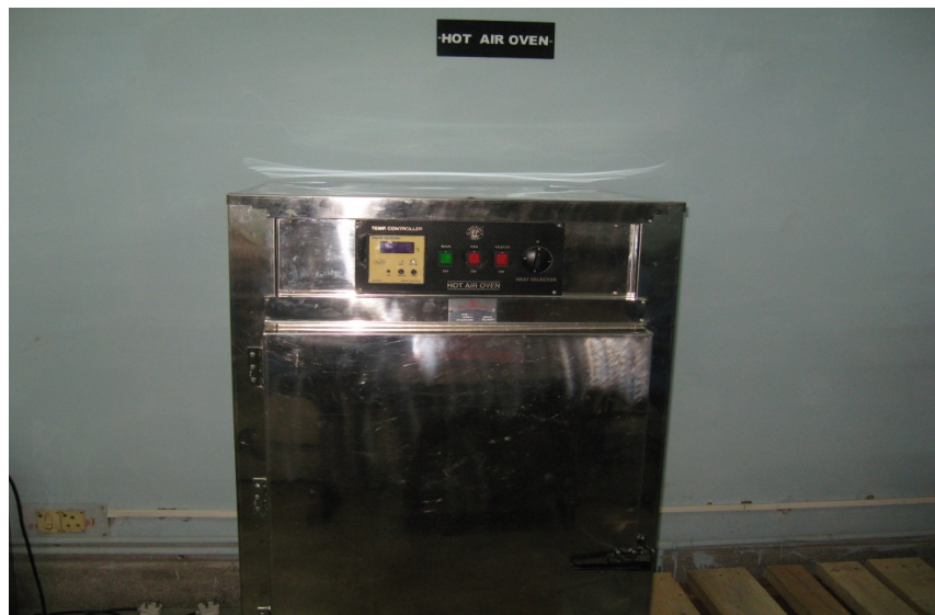
Plate A. 4.0: Hot air oven used for moisture content
