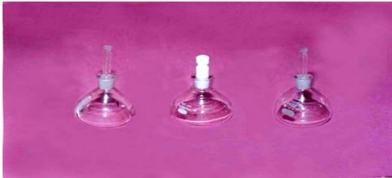
Plate 3.2 Pycnometers used for measurement of relative density
