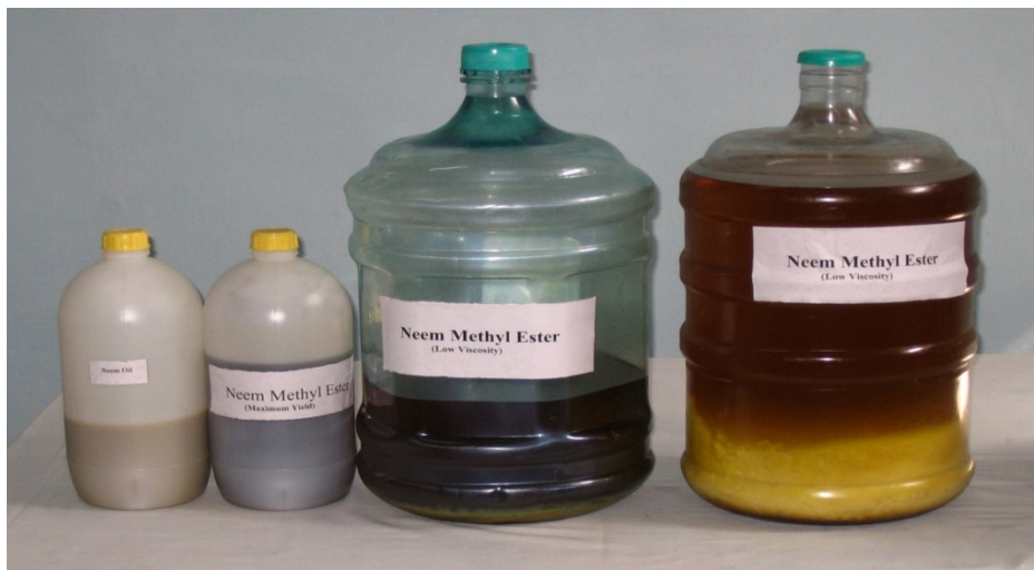
Plate 4.6 Neem methyl ester used for C.I. engine testing
