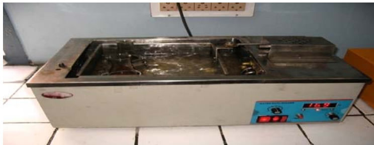
Plate 3.1 Water bath shaker for transesterification
