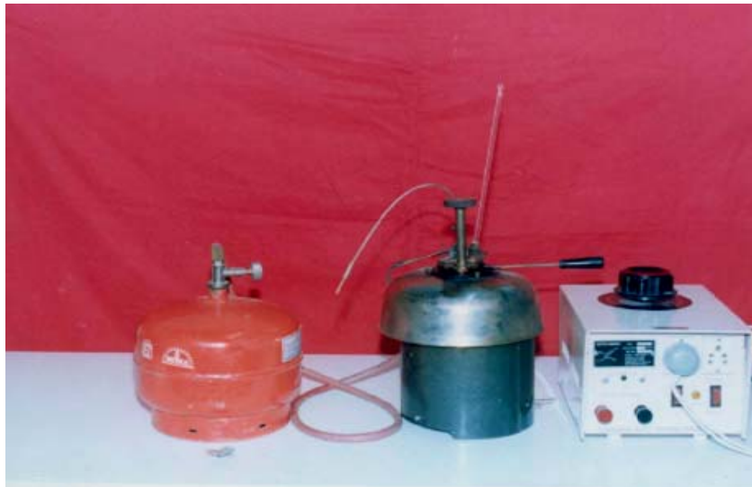
Plate 3.6 Pensky marten apparatus used for measurement of flash and fire point
