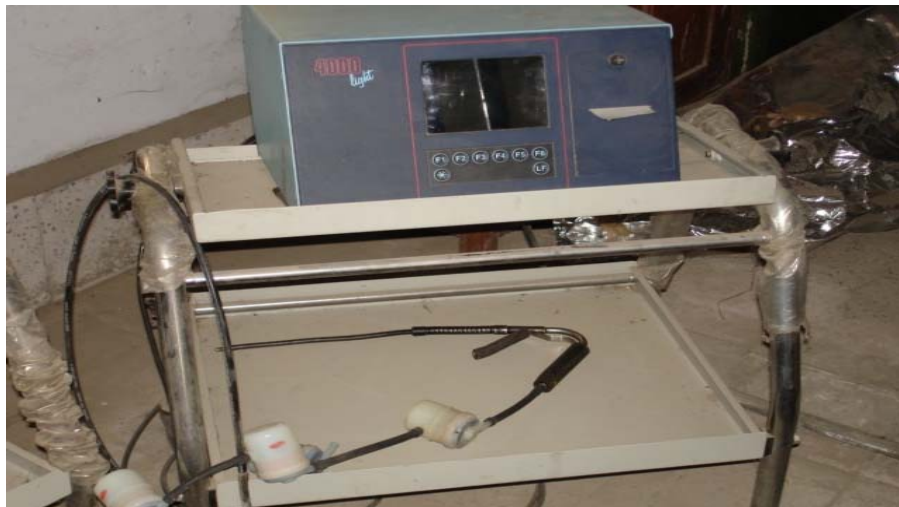
Plate 3.15 AVL Digas 4000 Five gas analyser used for NO x , CO 2 , UBHC, CO and O 2
