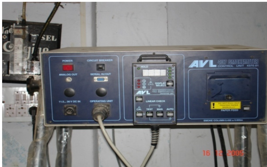
Plate 3.14 AVL smoke meter used for smoke opacity
