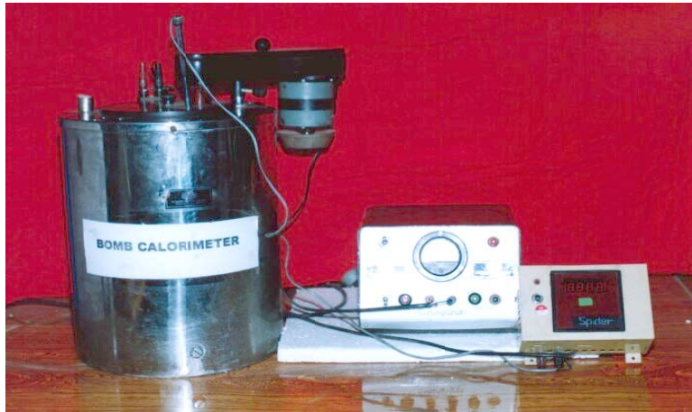
Plate 3.4 Isothermal bomb calorimeter used for measurement of calorific value
