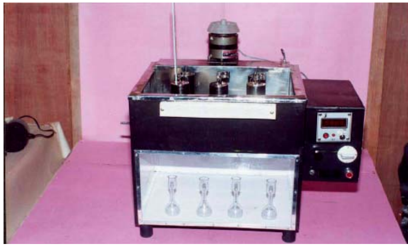
Plate 3.3 Redwood viscometer used for measurement of kinematic viscosity
