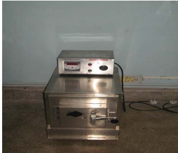
Plate A. 5. : Muffle furnace used for measurement of ash content
