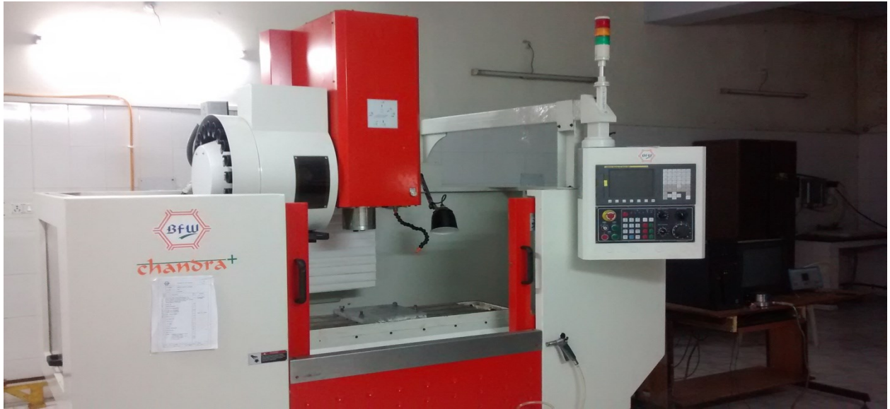
Figure 5.9: CNC vertical machining centre.
