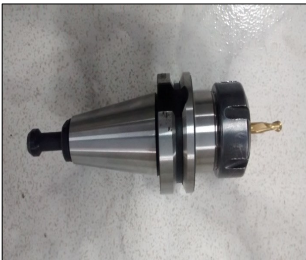
Figure 5.10.: Tool clamp with collate fixed with carbide tool.
