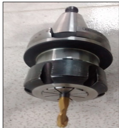
Figure 5.10.: Tool clamp with collate fixed with carbide tool.
