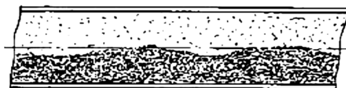
Figure 2.4: Strand flow (McGlinchey et al., 2007)
