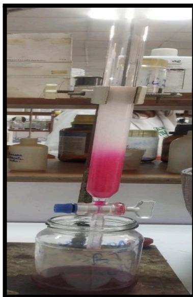
Figure 7. Purification of S. cumini anthocyanin extracts using Silica-Gel Column Chromatography
