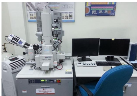
Figure 3.9 Laboratory Setup of FESEM [SAIF Lab, Panjab University, Chandigarh]
