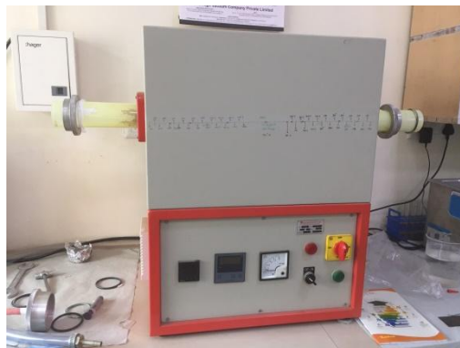
Figure 3.4: (a) Tubular Furnace [Thin Films Lab, Thapar University, Patiala]
