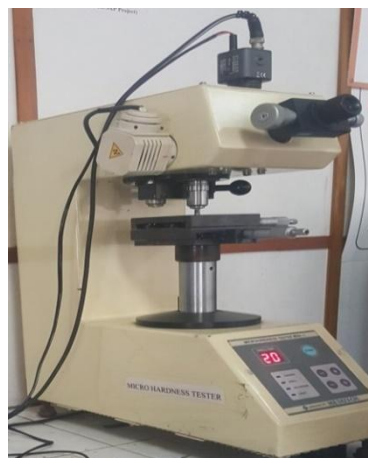
Figure 3.7: Micro Hardness Tester [Advanced Measurement Lab, Thapar University, Patiala]
