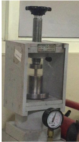
Figure 3.3: Manual Hydraulic Press [SPMS Lab, Thapar University, Patiala]
