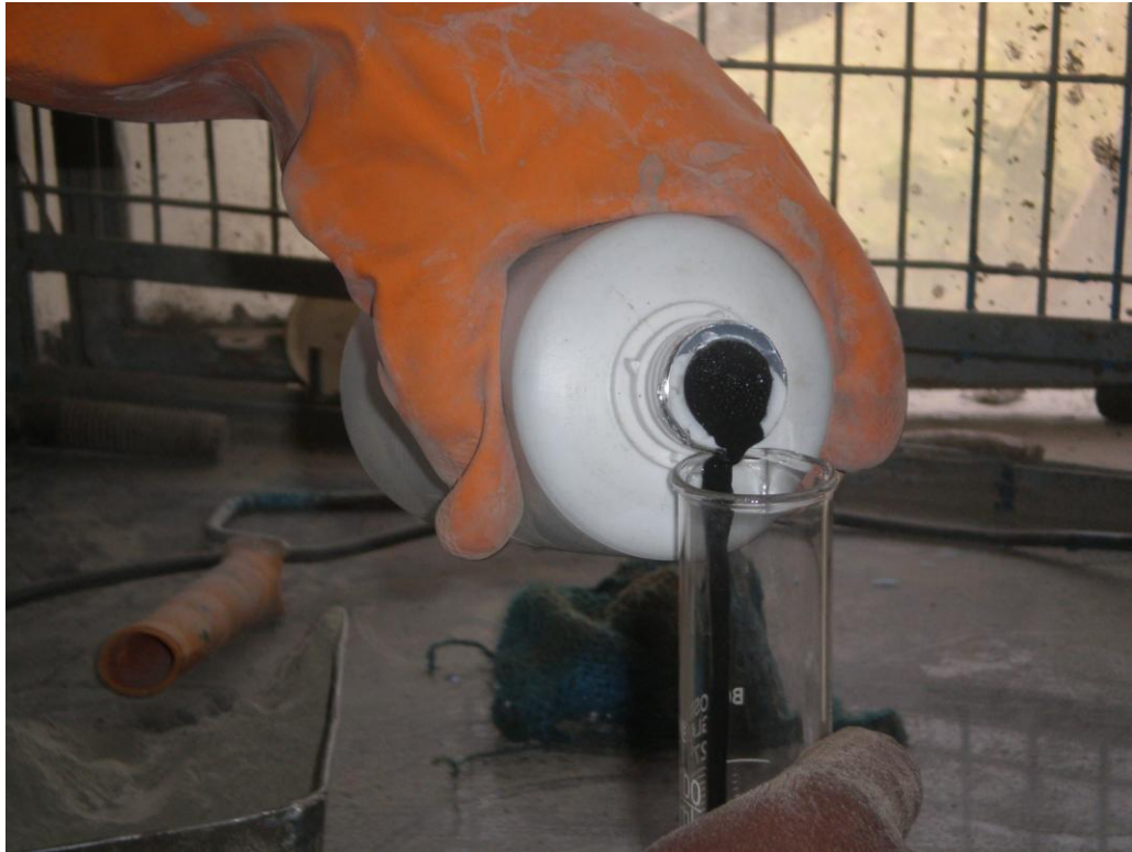
Fig. 3.3(c): Pouring of dispersed CNF in experiment
