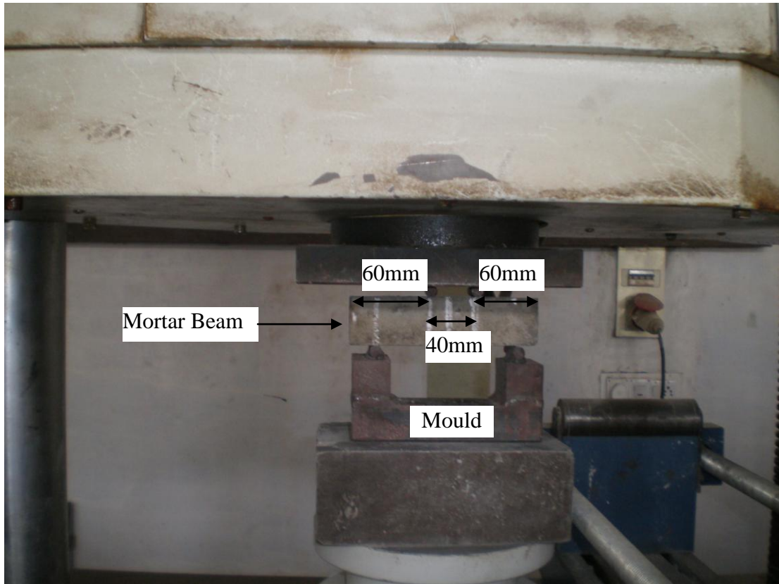
Figure 3.7: Beam under two point loading
