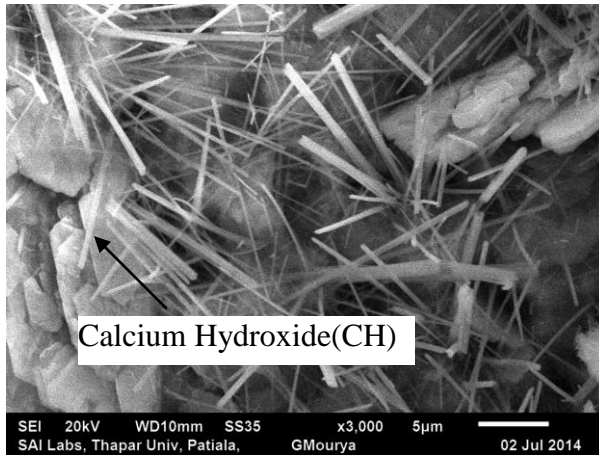
Figure 4.10(c): SEM micrograph of CNF 0.05% (7 days hydrated) showing Calcium Hydroxide
