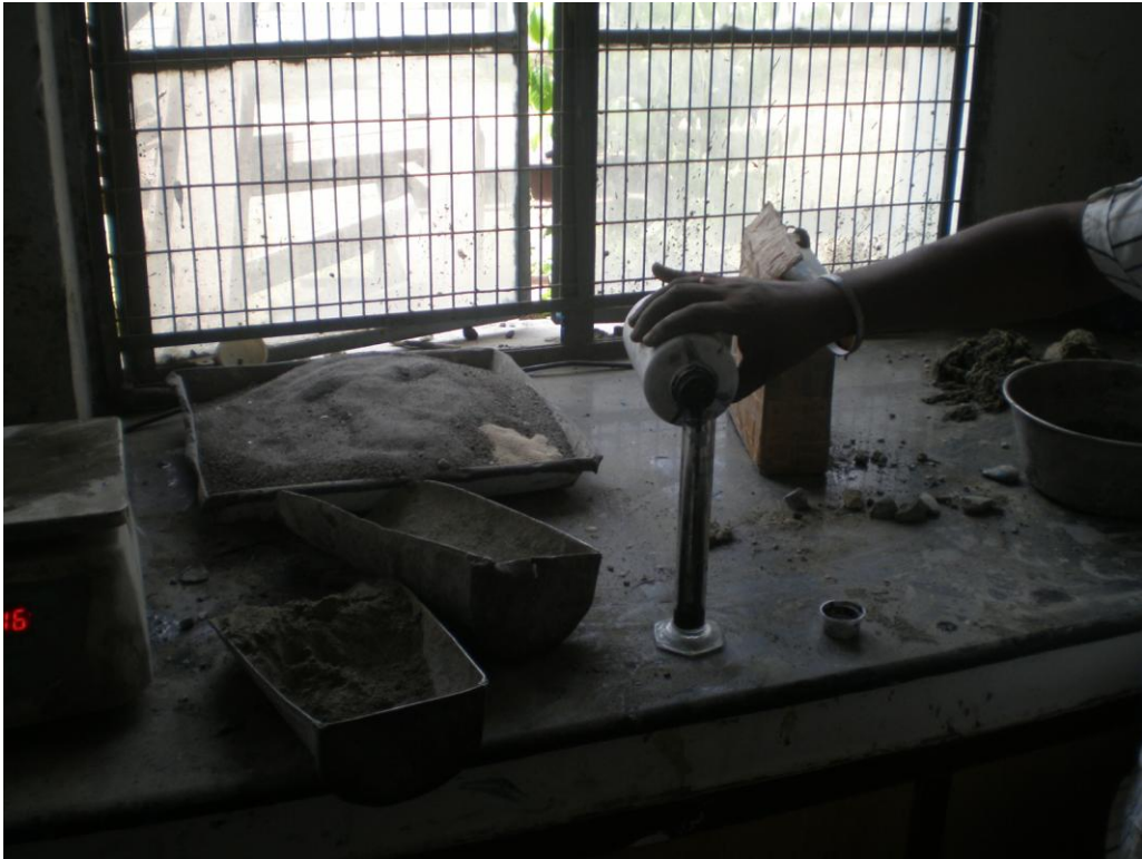
Figure 3.5: (a) Pouring of carbon fiber colloidal form during mixing of material
