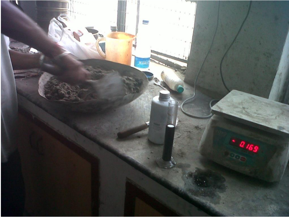
Figure 3.5: (c) Mixing of material for mortar cubes
