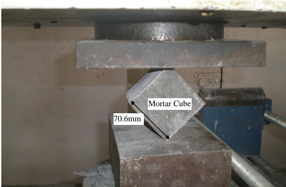
Figure 3.8: Cube under split tensile test
