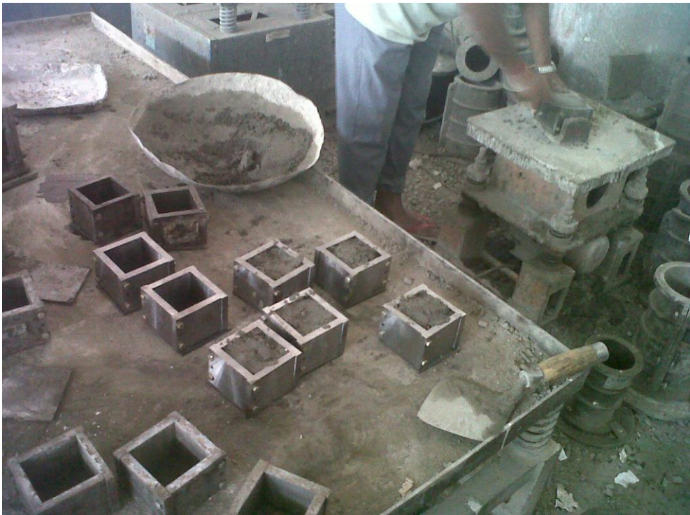
Figure 3.5: (d) Vibration of moulds filled by mortar in vibrating table
