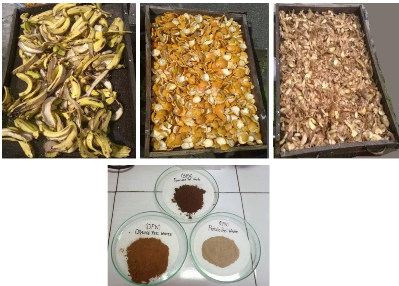
Fig. 34 Washed and air dried a) Banana peel, b) orange peel and c) potato peel d) powder form of biomass
