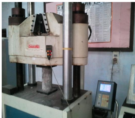
Fig 4.20 Compression Testing of Cube using UTM
