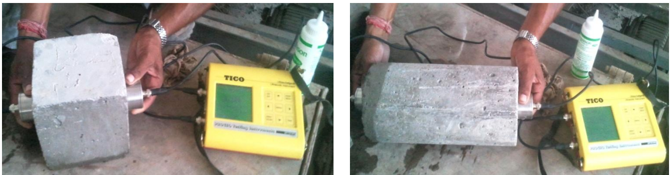
Fig 4.15(b) Second phase i.e. Hardening monitoring (During curing)
