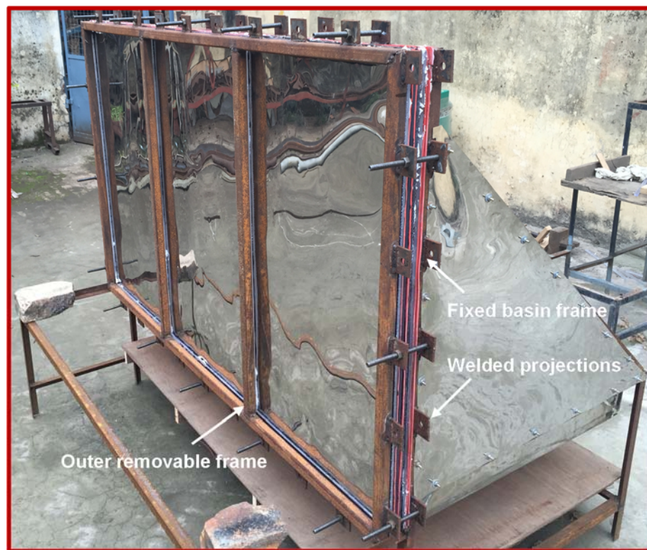
Fig. 3.6 Snapshot of distillation section frames with projections for nuts and bolts
