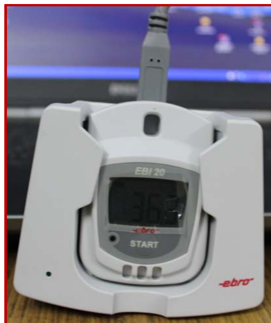
Fig. 3.12 Relative humidity meter
