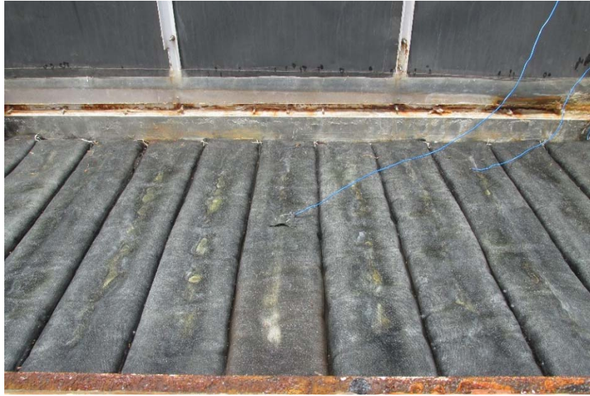
Fig. 4.37 Snapshot of cotton cloth wicks of floats showing salt deposition
