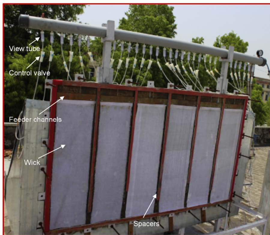
Fig. 3.7 Snapshot of partitioned wick structure in the FW-BVMED-HR still
