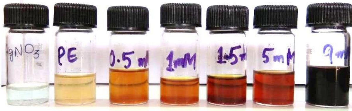
Figure 8: From left to right; \text{AgNO}_3 solution, Pineapple peel extract, \text{AgNO}_3 (0.5, 1, 1.5, 5, 9 mM) and peel extract mixture.
