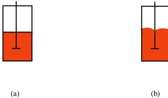
Fig. 2: The entrapment of air during stirring (a) before stirring (b) during stirring
