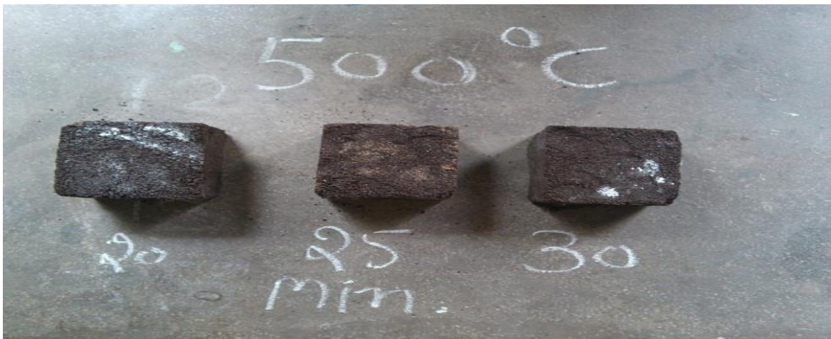
Figure 5.6 Samples of sand reclaimed at 500 °C for different time durations
