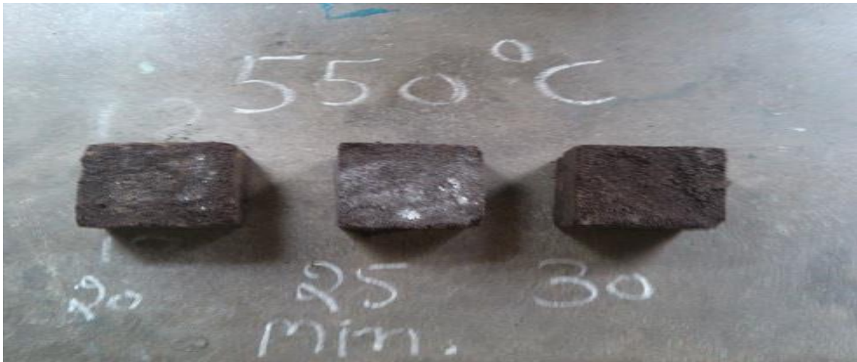
Figure 5.7 Samples of sand reclaimed at 550 °C for different time durations
