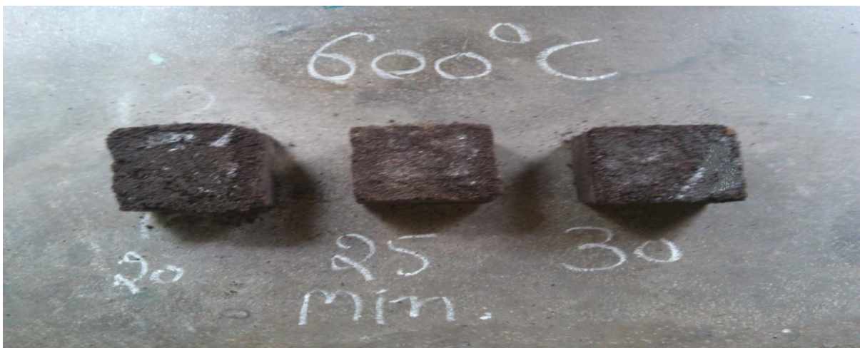
Figure 5.8 Samples of sand reclaimed at 600 °C for different time durations
