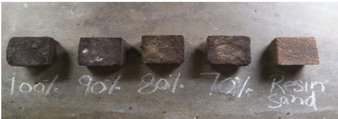
Figure 5.12 Reclaimed sand in different proportions with resin sand
