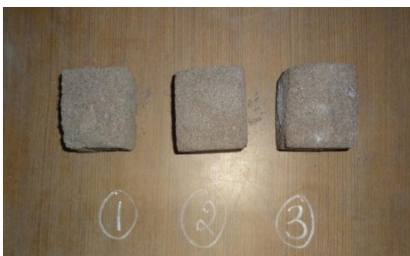
Figure 5.3 Resin coated core (75 mm square) specimen for testing
