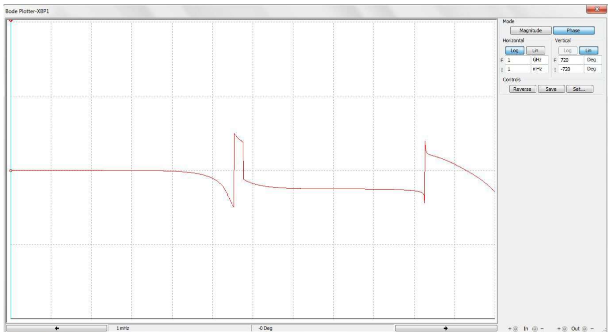
Figure 5.21: Phase Angle versus Frequency Response of Inverse Chebyshev LPF
