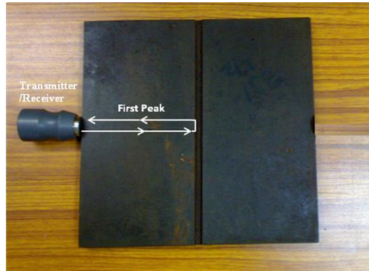
Figure 4.7: Pulse Echo of Plates Testing in Air
