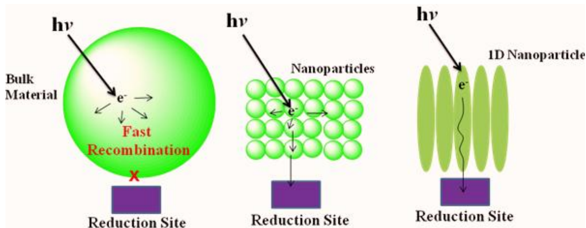
Fig. 1.2: Efficiency of 1D nanostructures over bulk and spherical particles due to axial electron transport.
