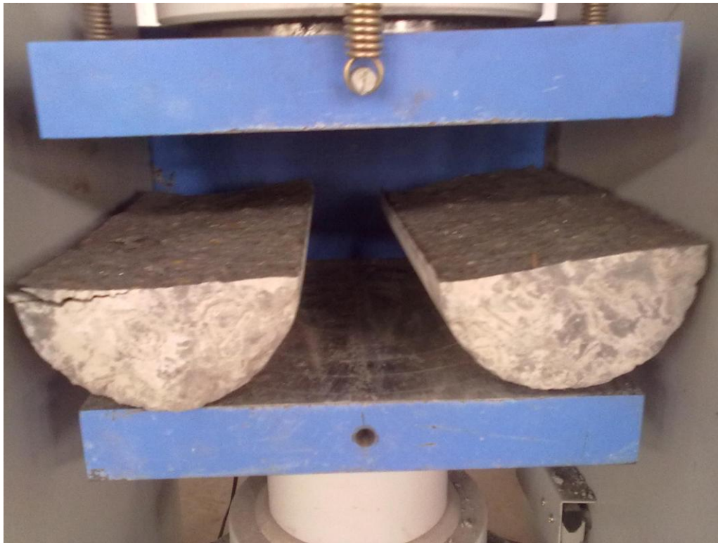
Fig. 5.7 : Splitting tensile strength test
