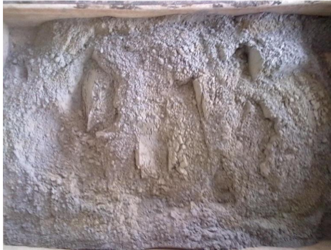
Fig. 4.1 : Silica Fume mixed with cement
