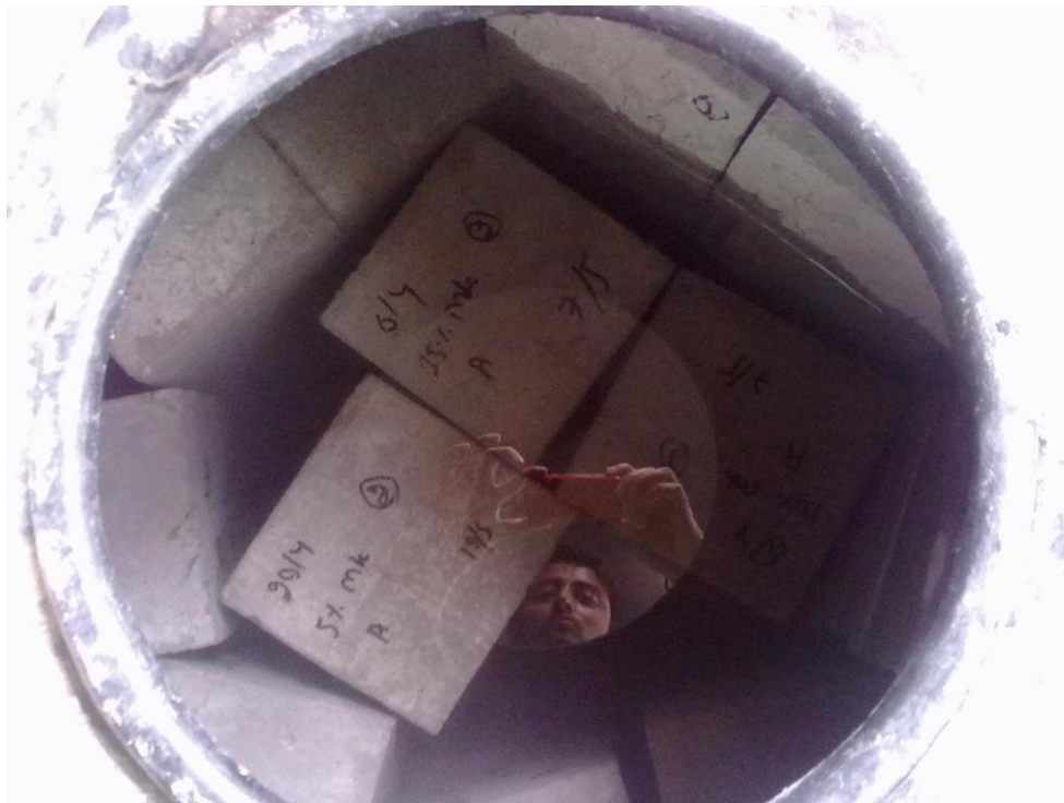
Fig. 5.8 : Cube specimen placed in 5% MgSO_4 solution (After 28 days initial curing)
