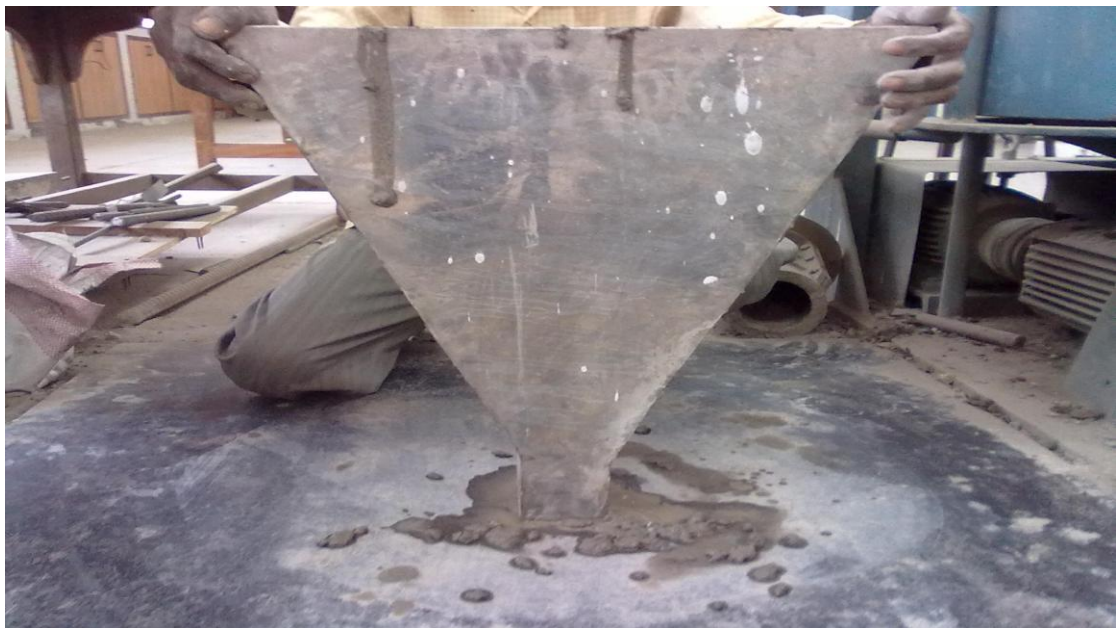
Fig. 5.2 : V Funnel Test
