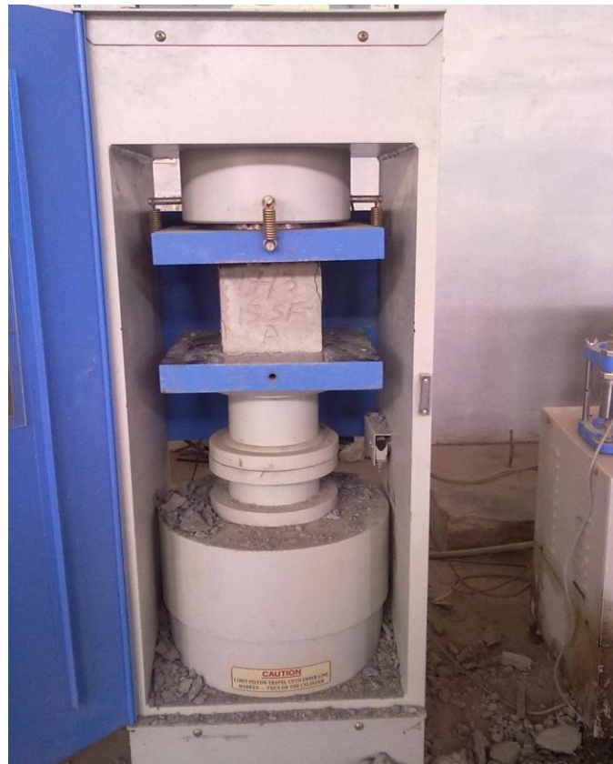
Fig. 5.5 : Compressive strength test in progress
