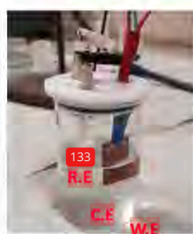
Fig. 2.4: Photograph of an electrochemical cell used for the EIS measurements
