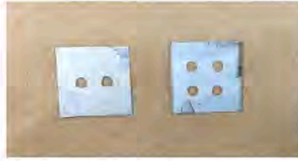
Fig. 2.2: Masks used during the deposition of the Al-contacts
