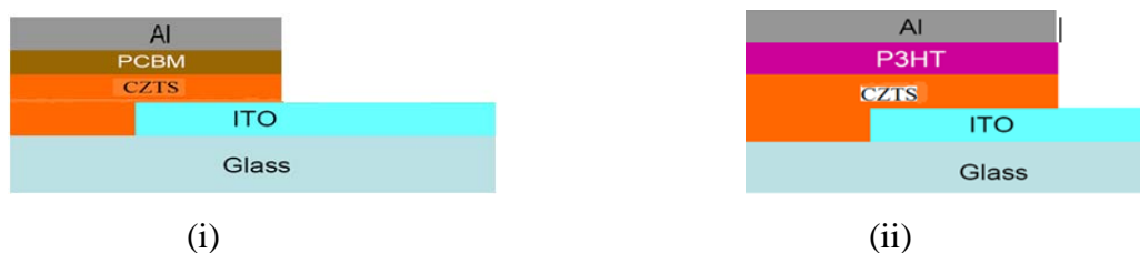
Figure 2.9: Scheme of a bilayer solar cell: ITO covered glass / CZTS layer (i) drop cast PCBM (ii) Drop cast P 3 HT layer /evaporated top electrode (Al).
